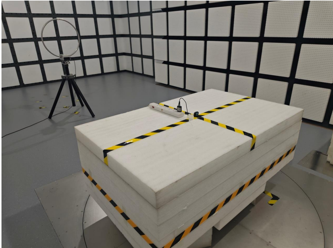
Radiated Emission 9 kHz-30 MHz Perpendicular View
