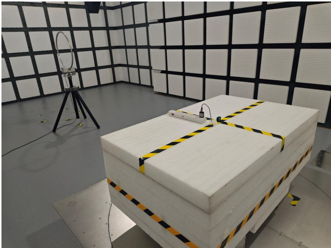
Radiated Emission 9 kHz-30 MHz Perpendicular View
