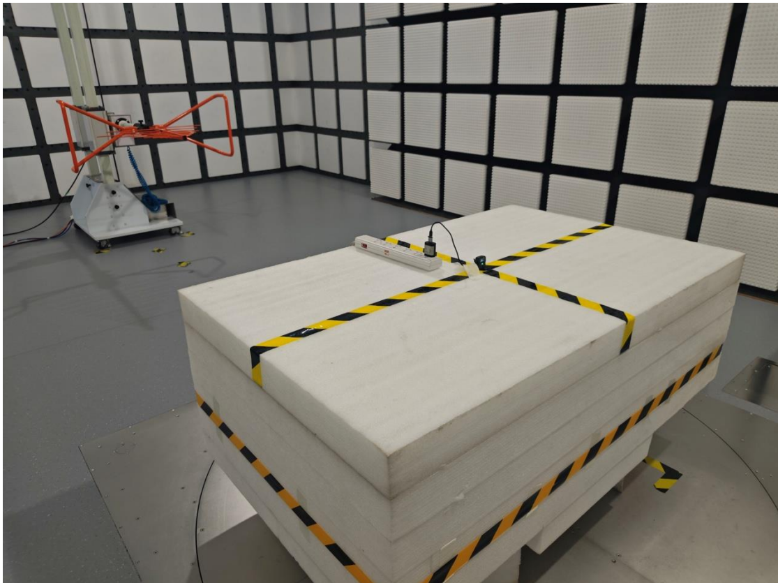
Radiated Emission 30 MHz-1 GHz View
