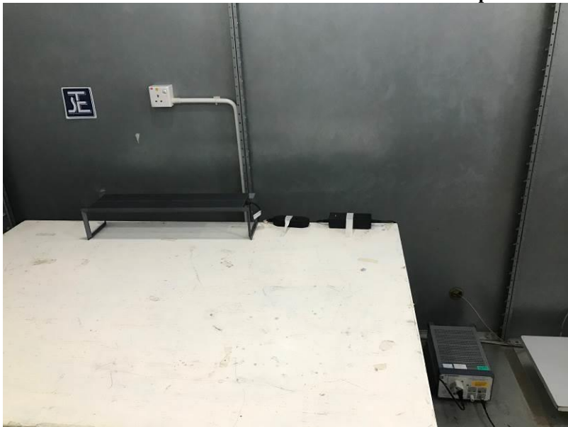
Measurement of Conducted Emission Test Set Up
