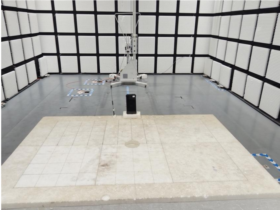
Radiated spurious emission Test Setup-2(Above 1GHz)
