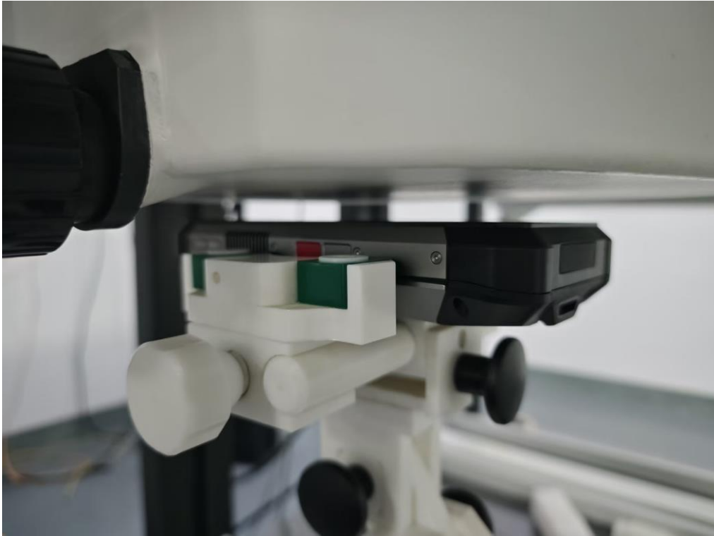
Body Front side (separation distance is 10mm)
