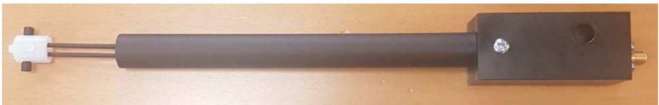
Figure 1 – MVG COMOSAR Validation Dipole
