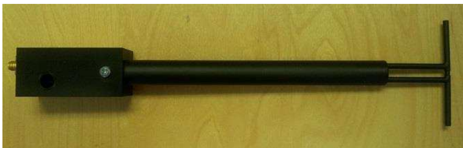
Figure 1 – MVG COMOSAR Validation Dipole
