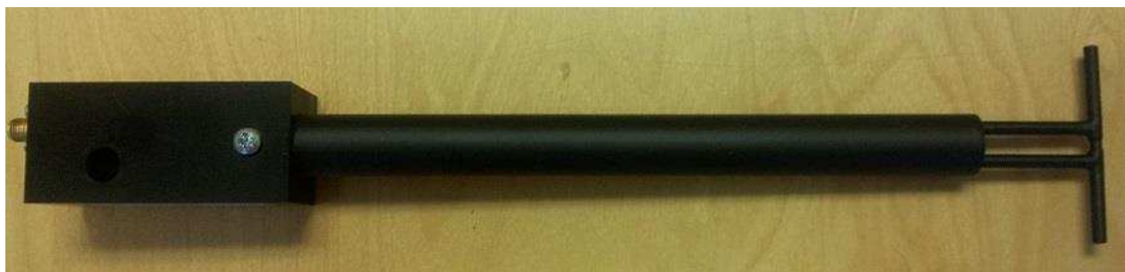
Figure 1 – MVG COMOSAR Validation Dipole
