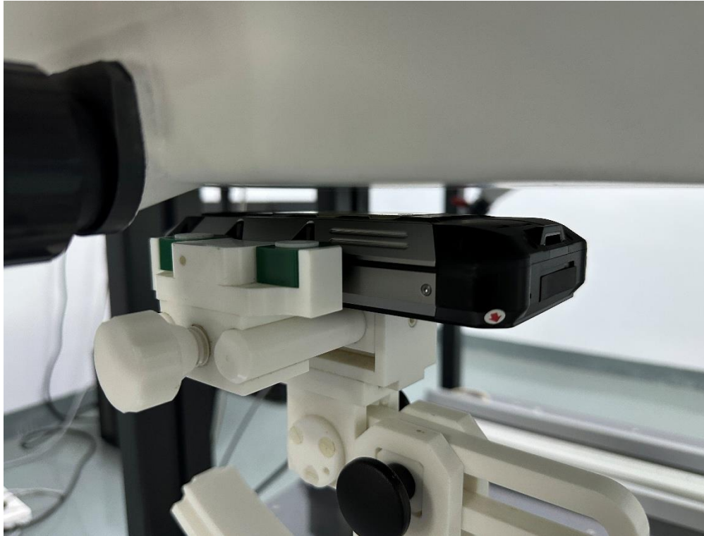
Body Back side (separation distance 10mm)
