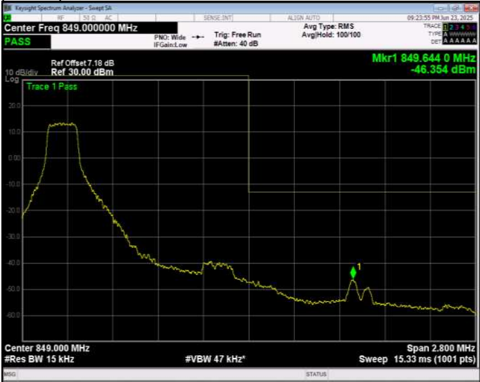
Band26(824-849) 16QAM BW=1.4MHz Channel=27033 RB Size=1 Position=#Max Normal
