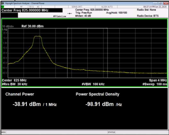
Band26(814-824) 16QAM BW=1.4MHz Channel=26783 RB Size=1 Position=#Max Extended
