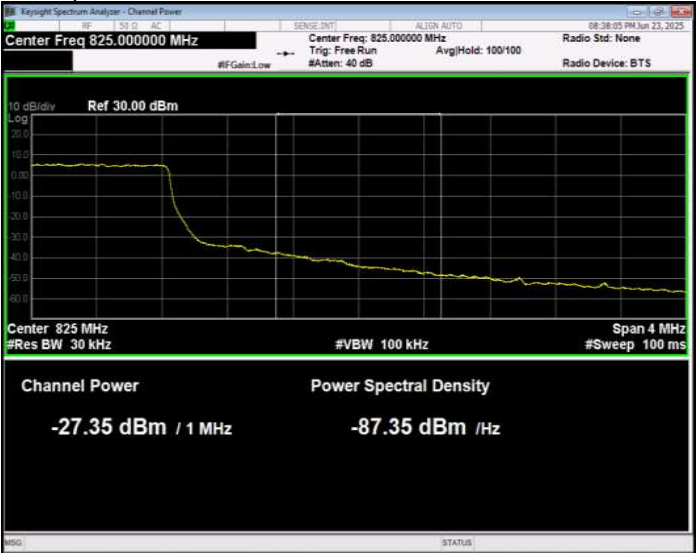
Band26(814-824) 16QAM BW=1.4MHz Channel=26783 RB Size=6 Position=#0 Normal
