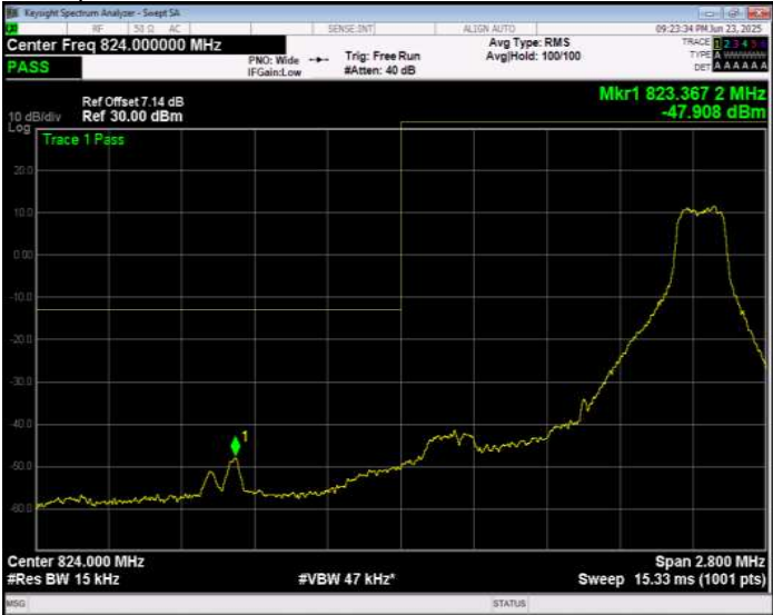
Band26(824-849) 16QAM BW=1.4MHz Channel=26797 RB Size=6 Position=#0 Normal
