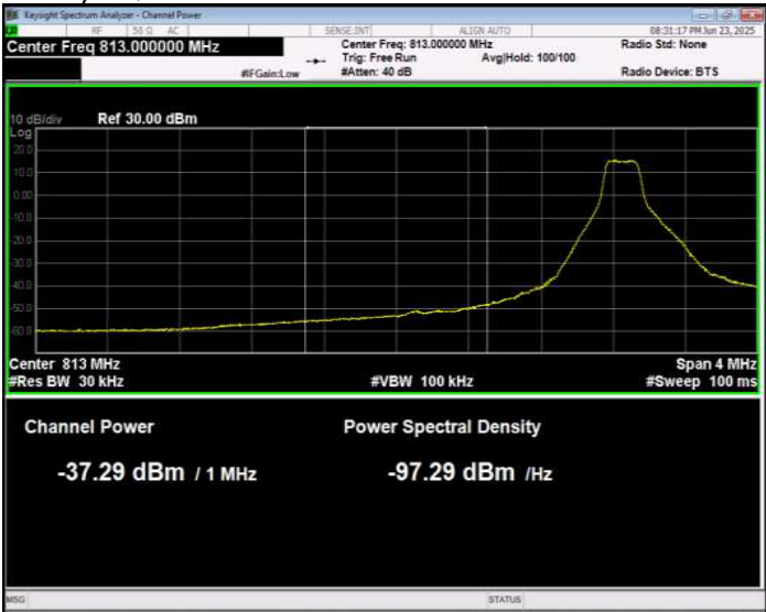
Band26(814-824) 16QAM BW=1.4MHz Channel=26697 RB Size=1 Position=#0 Normal
