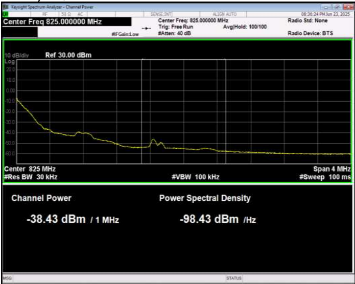
Band26(814-824) 16QAM BW=1.4MHz Channel=26783 RB Size=1 Position=#0 Normal
