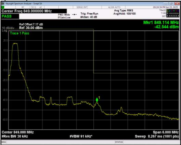
Band26(824-849) QPSK BW=3MHz Channel=27025 RB Size=1 Position=#Max Normal
