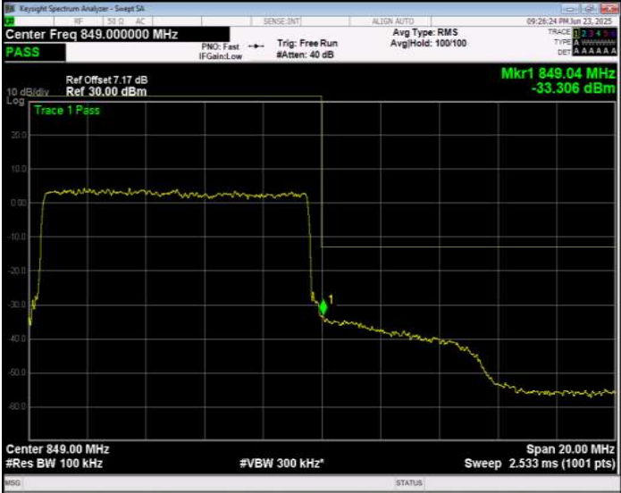
Band26(824-849) 16QAM BW=10MHz Channel=26990 RB Size=50 Position=#0 Normal
