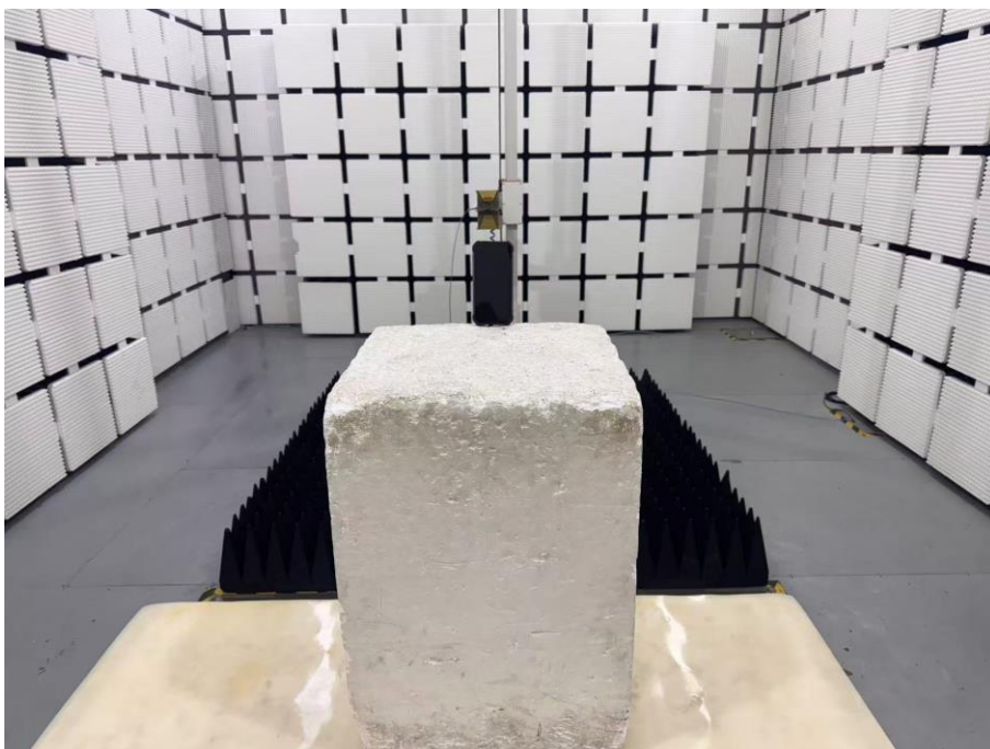
Set-up for Radiated Spurious Emission, Above 1GHz
