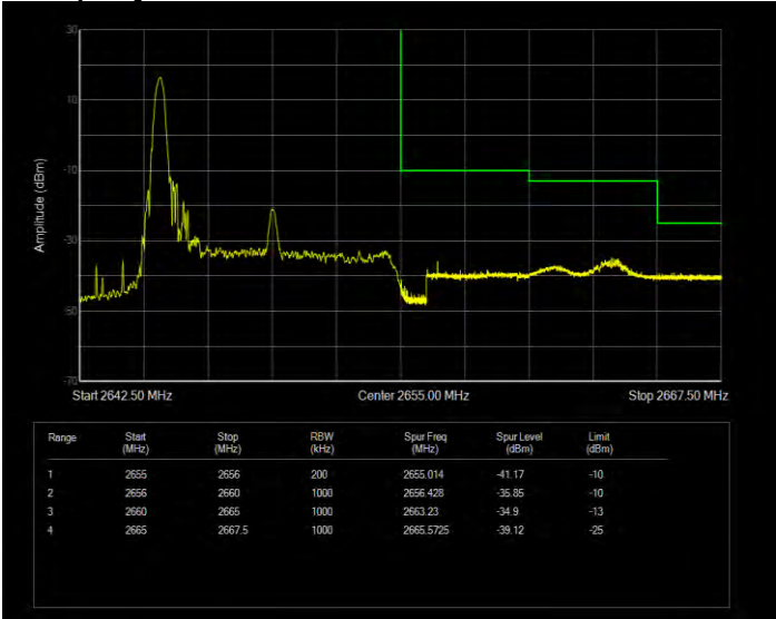
Band41(2555-2655) 16QAM BW=15MHz Channel=40315 RB Size=1 Position=#0 Extended
