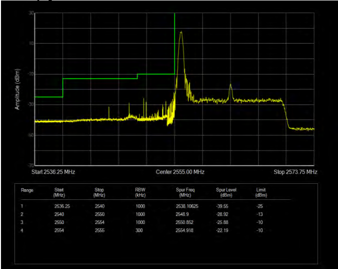
Band41(2555-2655) QPSK BW=15MHz Channel=41165 RB Size=1 Position=#0 Extended
