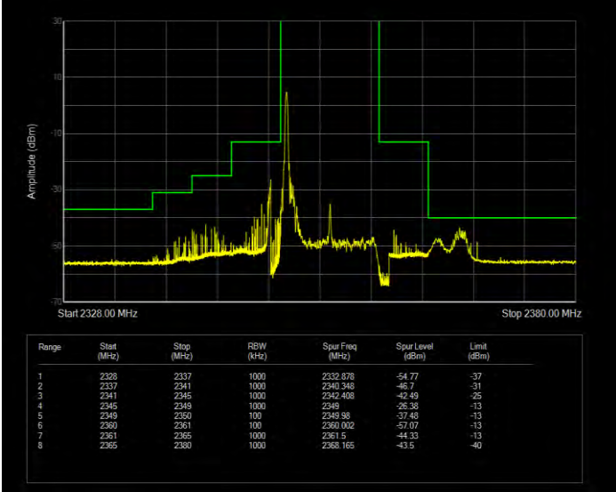
Band40(2350-2360) 16QAM BW=10MHz Channel=39200 RB Size=50 Position=#0 Extended
