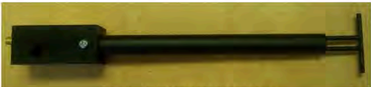
Figure 1 – MVG COMOSAR Validation Dipole
