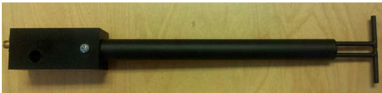
Figure 1 – MVG COMOSAR Validation Dipole
