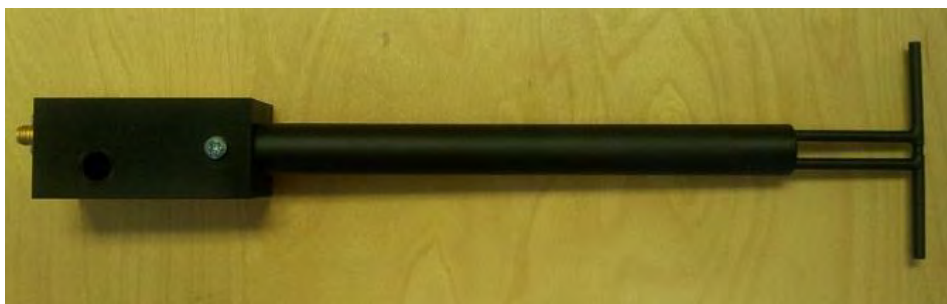
Figure 1 – MVG COMOSAR Validation Dipole
