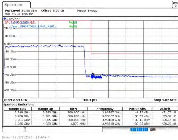
n77(3700-3980) SCS=30kHz DFT_QPSK BW=40MHz HighChannel=664000 RB=100@0
