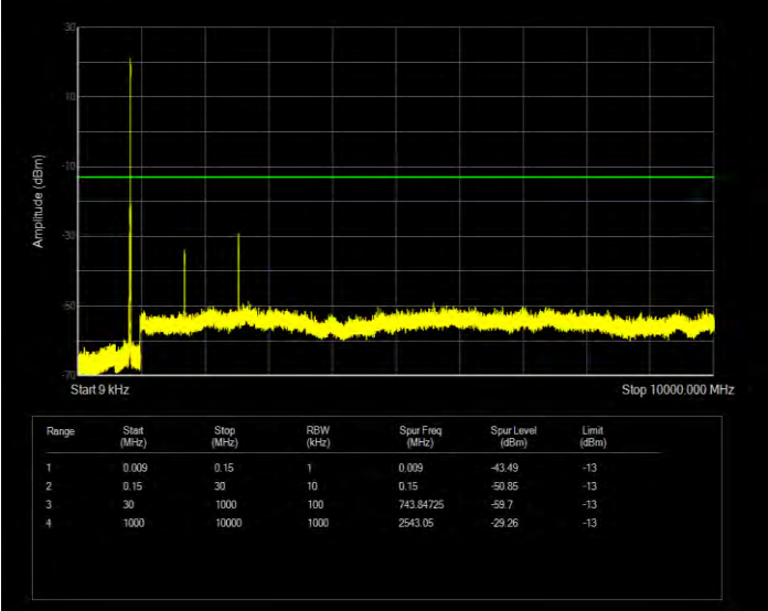
Band26(824-849) QPSK BW=5MHz Channel=26815 RB Size=25 Position=#0
