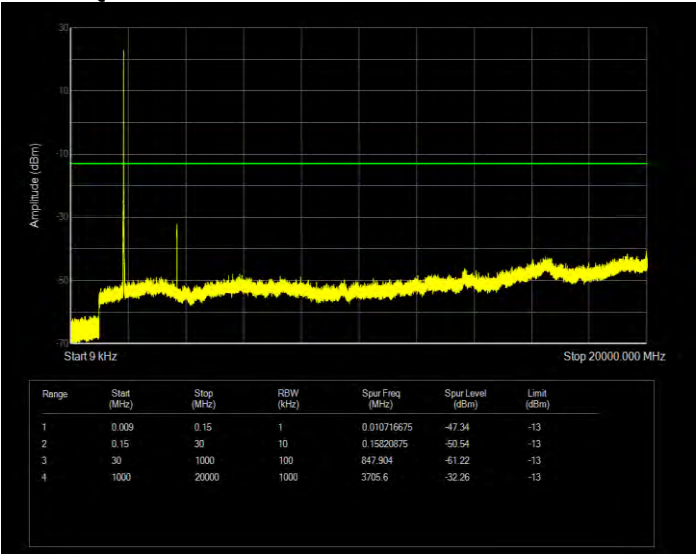
Band25 16QAM BW=5MHz Channel=26065 RB Size=25 Position=#0
