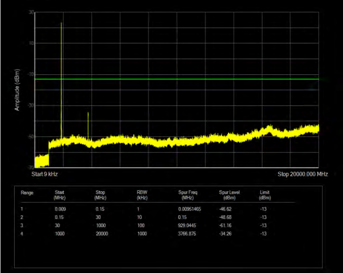
Band25 16QAM BW=3MHz Channel=26675 RB Size=15 Position=#0
