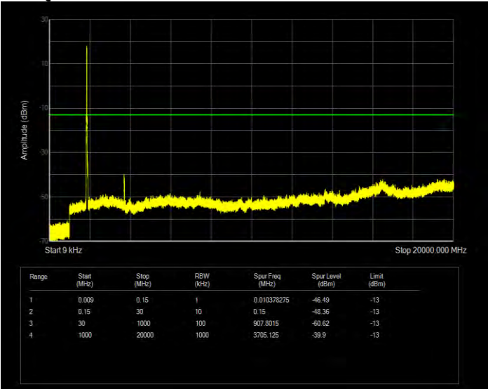
Band25 QPSK BW=20MHz Channel=26140 RB Size=100 Position=#0
