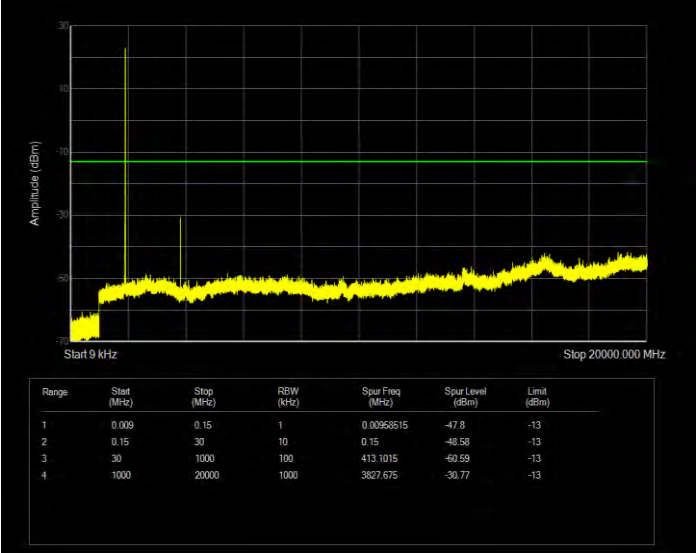
Band25 16QAM BW=5MHz Channel=26065 RB Size=25 Position=#0
