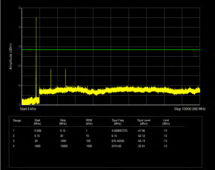
Band26(824-849) 16QAM BW=1.4MHz Channel=26915 RB Size=6 Position=#0
