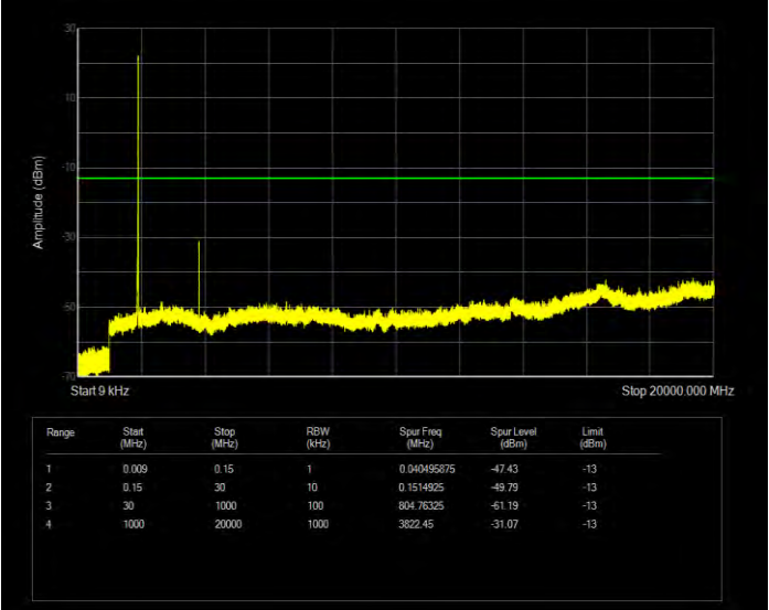
Band25 QPSK BW=1.4MHz Channel=26047 RB Size=6 Position=#0
