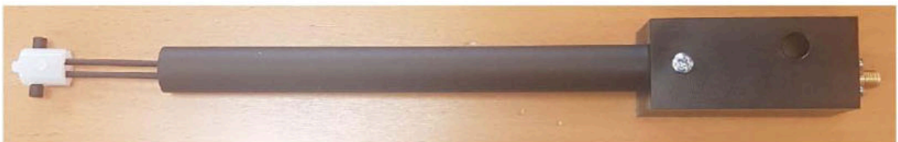
Figure 1 – MVG COMOSAR Validation Dipole
