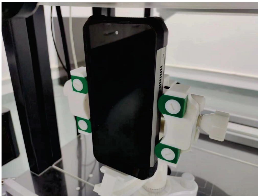
Body Top side (separation distance is 10mm)
