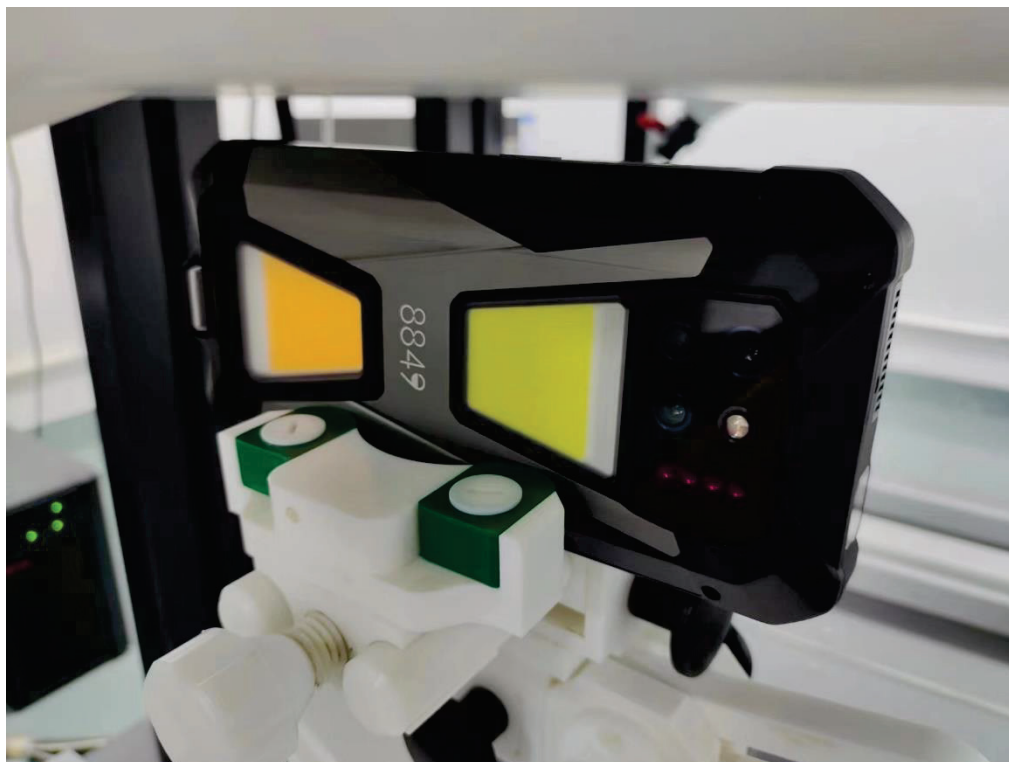
Body Right side (separation distance is 10mm)
