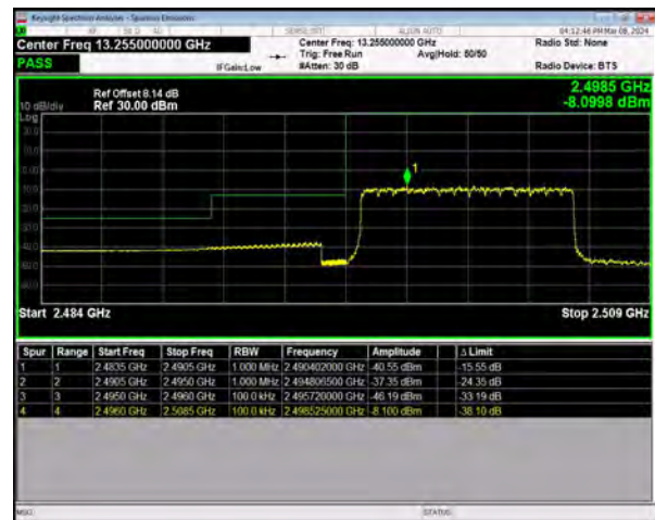
n41 SCS=30kHz DFT_256QAM BW=10MHz LowChannel=500202 RB=24@0
