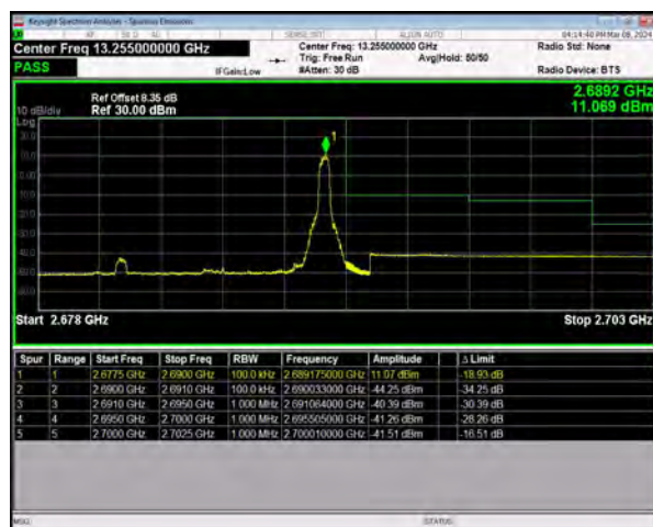
n41 SCS=30kHz DFT_QPSK BW=10MHz HighChannel=537000 RB=1@23
