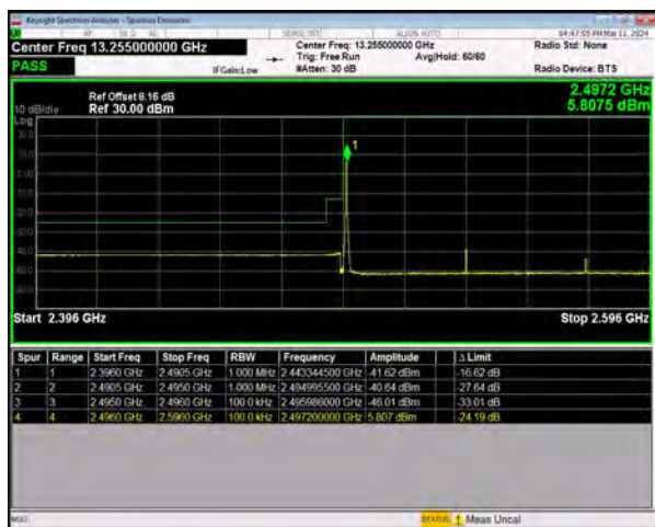
n41 SCS=30kHz DFT_16QAM BW=80MHz LowChannel=507204 RB=1@0
