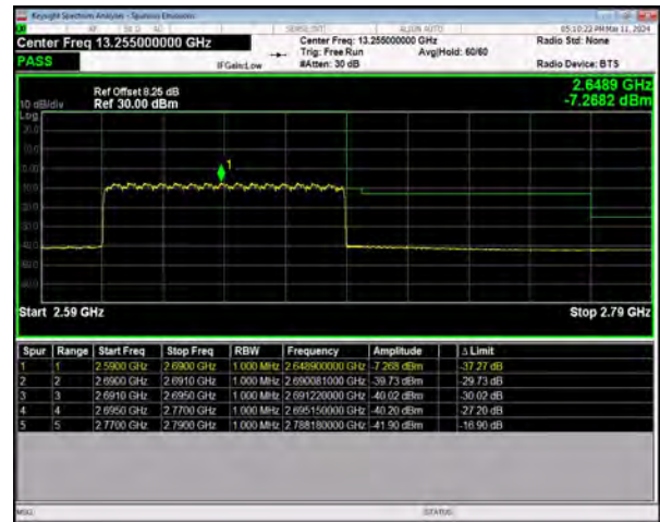
n41 SCS=30kHz CP_QPSK BW=80MHz HighChannel=529998 RB=217@0
