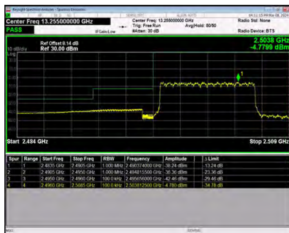
n41 SCS=30kHz DFT_16QAM BW=10MHz LowChannel=500202 RB=24@0
