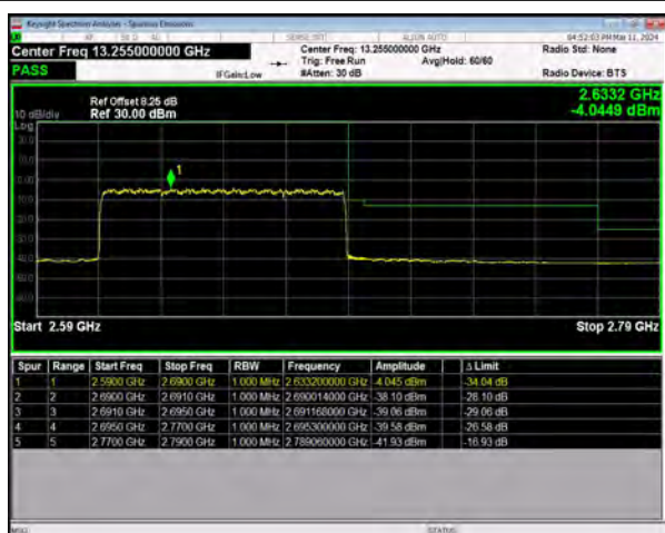
n41 SCS=30kHz DFT_BPSK BW=80MHz HighChannel=529998
