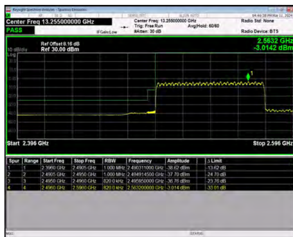
n41 SCS=30kHz DFT_QPSK BW=80MHz LowChannel=507204 RB=216@0
