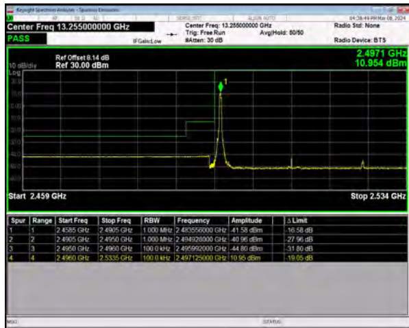
n41 SCS=30kHz DFT_BPSK BW=30MHz LowChannel=502200 RB=1@0
