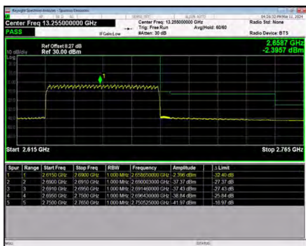
n41 SCS=30kHz DFT_QPSK BW=60MHz HighChannel=531996 RB=162@0
