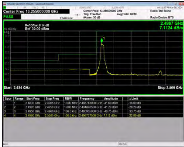
n41 SCS=30kHz DFT_64QAM BW=10MHz LowChannel=500202 RB=1@0
