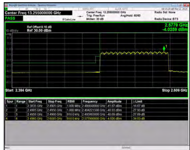
n41 SCS=30kHz DFT_BPSK BW=90MHz LowChannel=508200 RB=240@0
