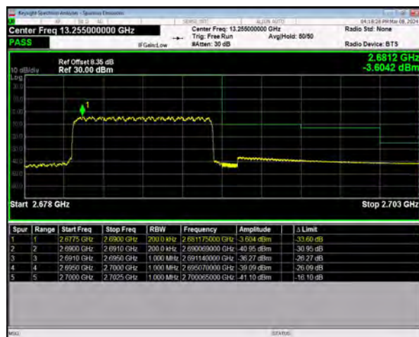
n41 SCS=30kHz CP_QPSK BW=10MHz HighChannel=537000
