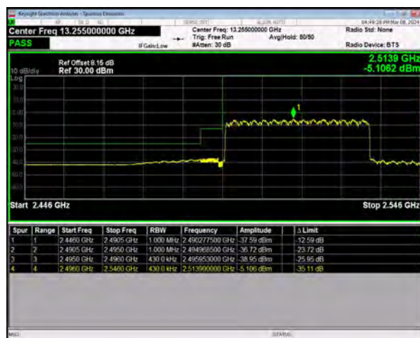
n41 SCS=30kHz DFT_QPSK BW=40MHz LowChannel=503202 RB=100@0
