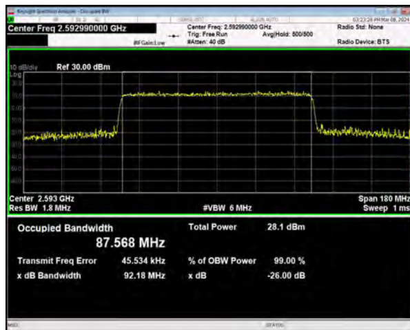
n41 SCS=30kHz CP_64QAM BW=90MHz Channel=518598 RB=245@0
