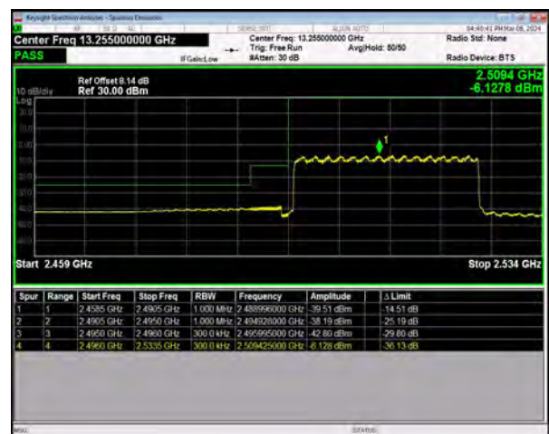
n41 SCS=30kHz DFT_16QAM BW=30MHz LowChannel=502200 RB=75@0
