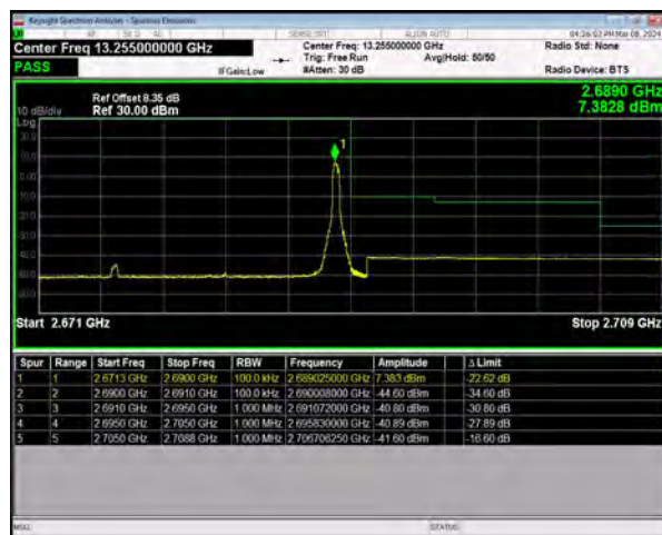
n41 SCS=30kHz DFT_64QAM BW=15MHz HighChannel=536496 RB=1@37
