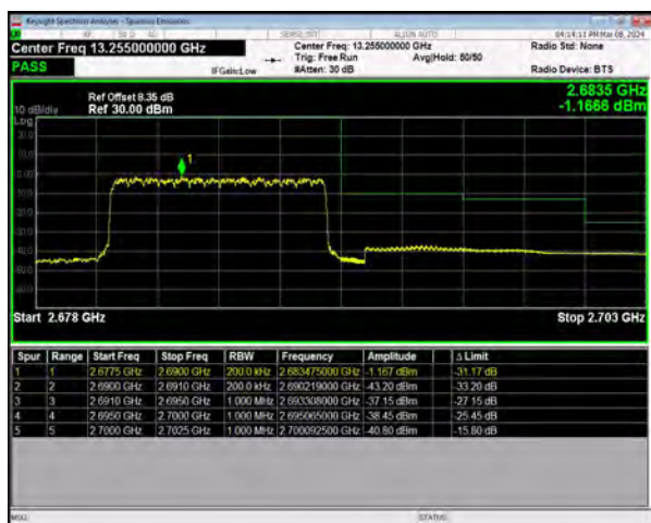
n41 SCS=30kHz DFT_BPSK BW=10MHz HighChannel=537000 RB=24@0
