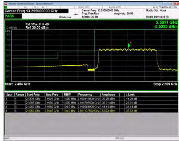
n41 SCS=30kHz DFT_64QAM BW=10MHz LowChannel=500202 RB=24@0
