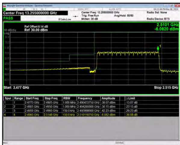
n41 SCS=30kHz CP_QPSK BW=15MHz LowChannel=500700
