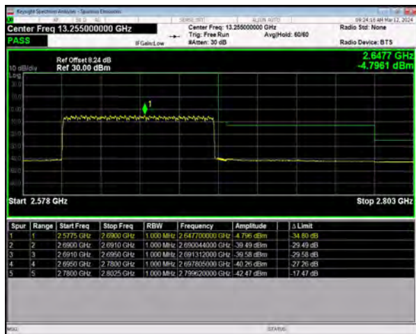
n41 SCS=30kHz DFT_BPSK BW=90MHz HighChannel=528996 RB=240@0
