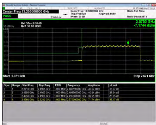
n41 SCS=30kHz CP_QPSK BW=100MHz LowChannel=509202
