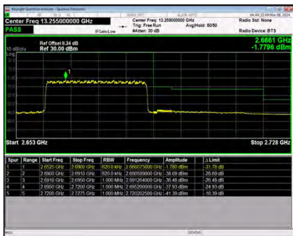
n41 SCS=30kHz DFT_QPSK BW=30MHz HighChannel=534996 RB=75@0
