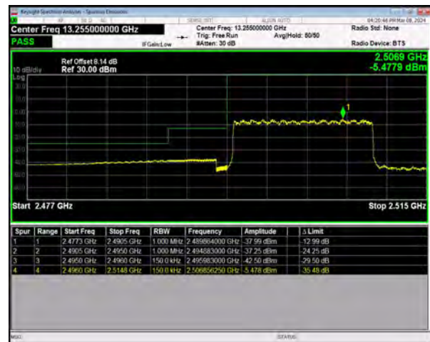
n41 SCS=30kHz DFT_16QAM BW=15MHz LowChannel=500700 RB=36@0
