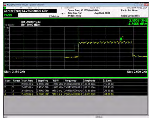
n41 SCS=30kHz DFT_QPSK BW=90MHz LowChannel=508200 RB=240@0
