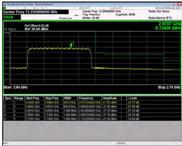
n41 SCS=30kHz DFT_QPSK BW=40MHz HighChannel=534000 RB=100@0
