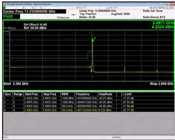
n41 SCS=30kHz DFT_16QAM BW=90MHz LowChannel=508200 RB=1@0
