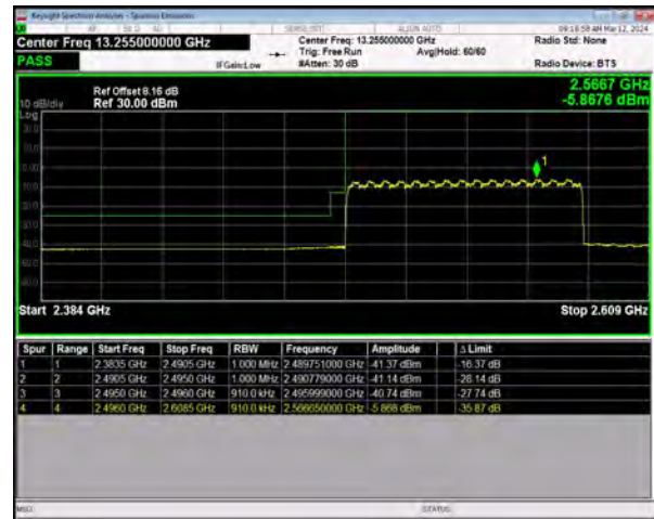
n41 SCS=30kHz DFT_16QAM BW=90MHz LowChannel=508200 RB=240@0
