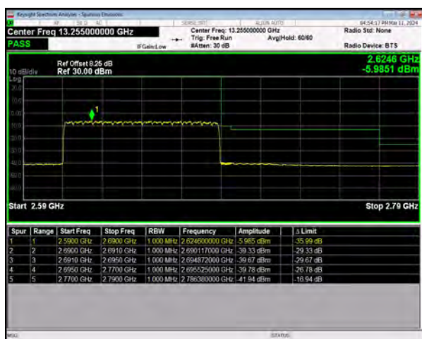
n41 SCS=30kHz DFT_16QAM BW=80MHz HighChannel=529998 RB=216@0
