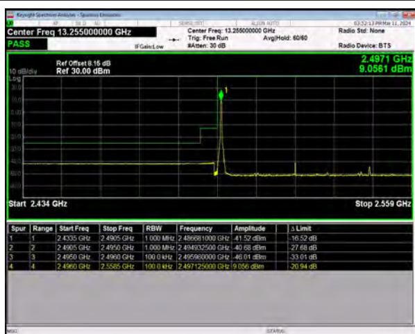
n41 SCS=30kHz DFT_QPSK BW=50MHz LowChannel=504204 RB=1@0
