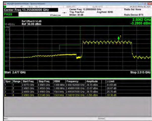
n41 SCS=30kHz DFT_QPSK BW=15MHz LowChannel=500700 RB=36@0
