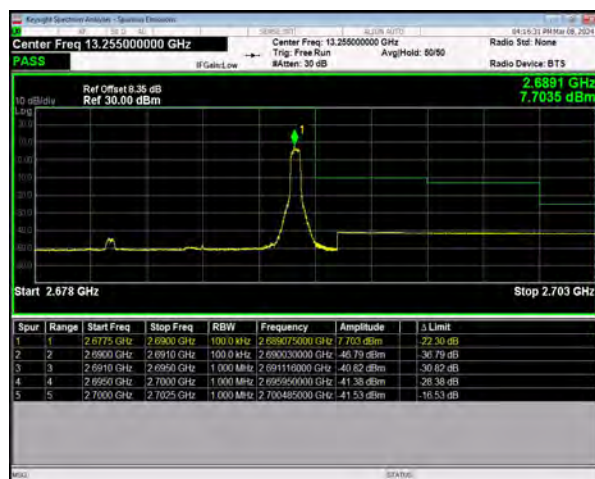
n41 SCS=30kHz DFT_64QAM BW=10MHz HighChannel=537000 RB=1@23
