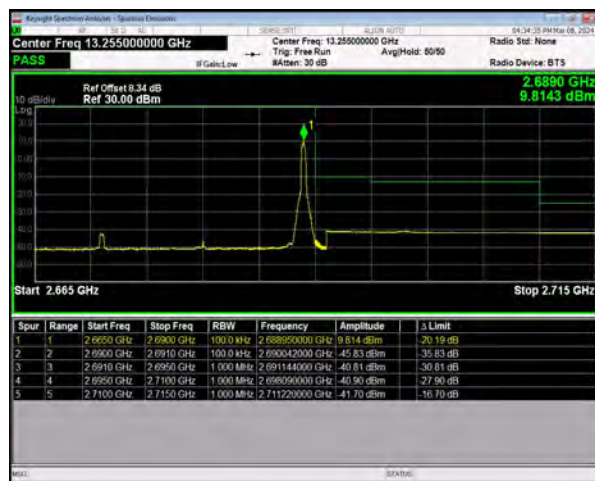
n41 SCS=30kHz DFT_QPSK BW=20MHz HighChannel=535998 RB=1@50
