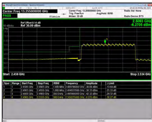
n41 SCS=30kHz CP_QPSK BW=30MHz LowChannel=502200
