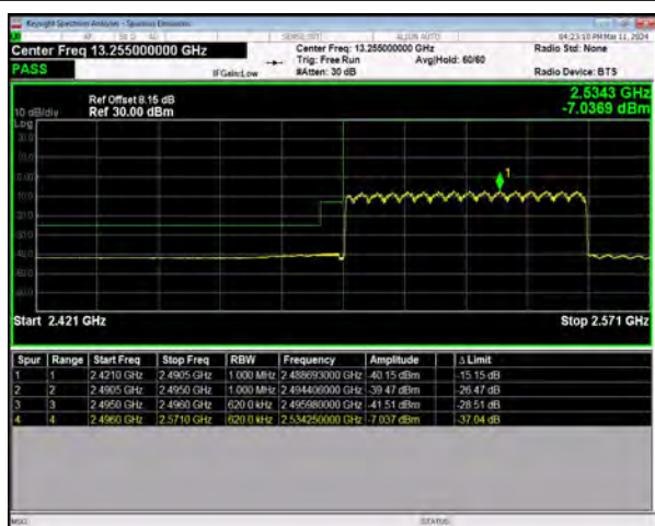
n41 SCS=30kHz CP_QPSK BW=60MHz LowChannel=505200
