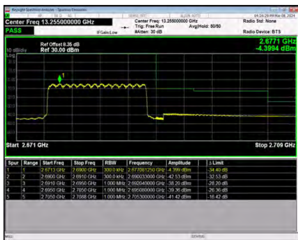
n41 SCS=30kHz DFT_64QAM BW=15MHz HighChannel=536496 RB=36@0
