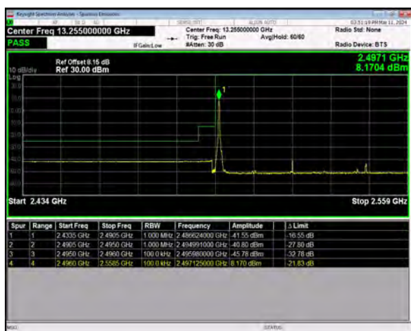
n41 SCS=30kHz DFT_BPSK BW=50MHz LowChannel=504204 RB=1@0
