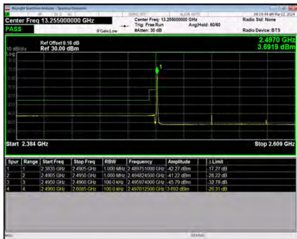
n41 SCS=30kHz DFT_64QAM BW=90MHz LowChannel=508200 RB=1@0
