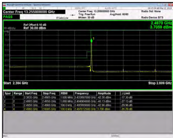
n41 SCS=30kHz DFT_BPSK BW=90MHz LowChannel=508200 RB=1@0
