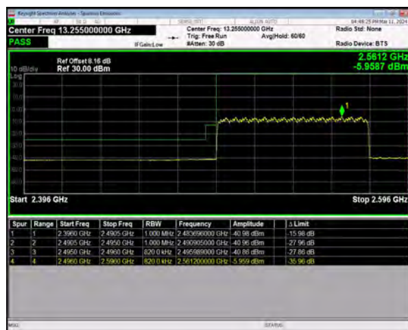
n41 SCS=30kHz DFT_64QAM BW=80MHz LowChannel=507204 RB=216@0
