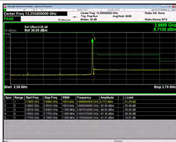
n41 SCS=30kHz DFT_QPSK BW=80MHz HighChannel=529998
