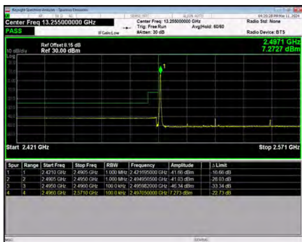
n41 SCS=30kHz DFT_16QAM BW=60MHz LowChannel=505200 RB=1@0
