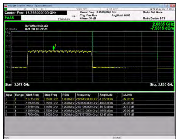
n41 SCS=30kHz CP_QPSK BW=90MHz HighChannel=528996 RB=245@0
