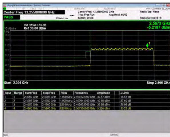
n41 SCS=30kHz DFT_16QAM BW=80MHz LowChannel=507204 RB=216@0
