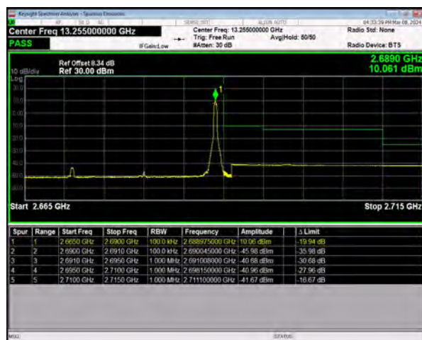
n41 SCS=30kHz DFT_BPSK BW=20MHz HighChannel=535998 RB=1@50
