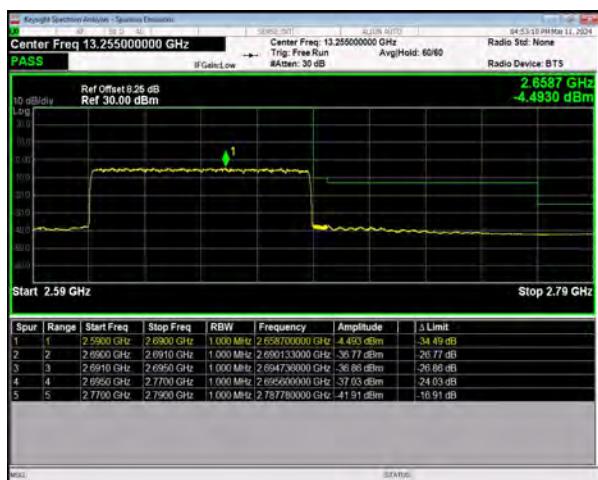
n41 SCS=30kHz DFT_QPSK BW=80MHz HighChannel=529998 RB=216@0
