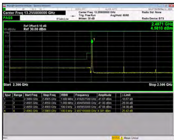
n41 SCS=30kHz DFT_64QAM BW=80MHz LowChannel=507204 RB=1@0
