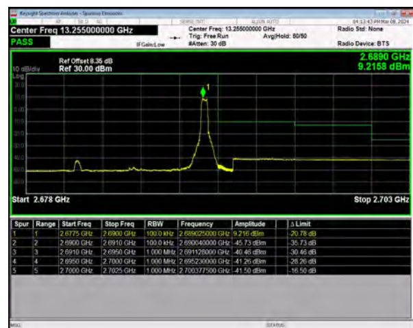
n41 SCS=30kHz DFT_BPSK BW=10MHz HighChannel=537000 RB=1@23
