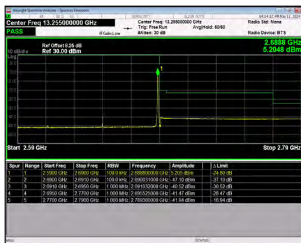
n41 SCS=30kHz DFT_64QAM BW=80MHz HighChannel=529998 RB=1@216
