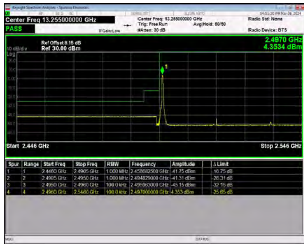
n41 SCS=30kHz DFT_256QAM BW=40MHz LowChannel=503202 RB=1@0
