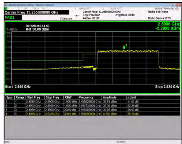
n41 SCS=30kHz DFT_QPSK BW=30MHz LowChannel=502200 RB=75@0
