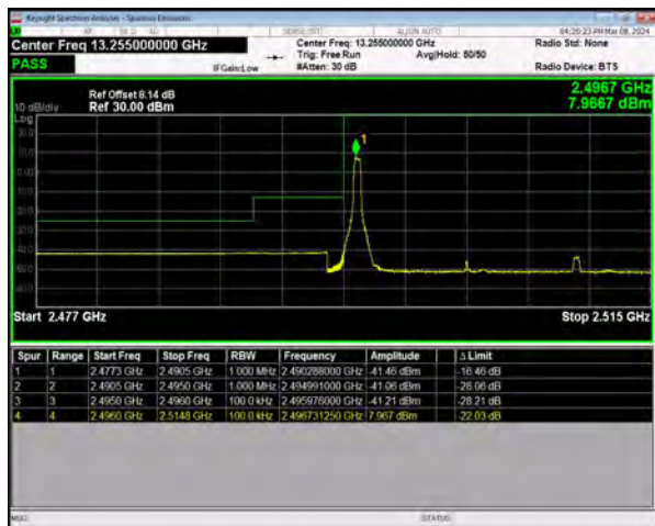
n41 SCS=30kHz DFT_16QAM BW=15MHz LowChannel=500700 RB=1@0
