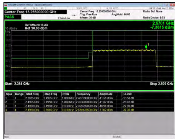
n41 SCS=30kHz DFT_64QAM BW=90MHz LowChannel=508200 RB=240@0
