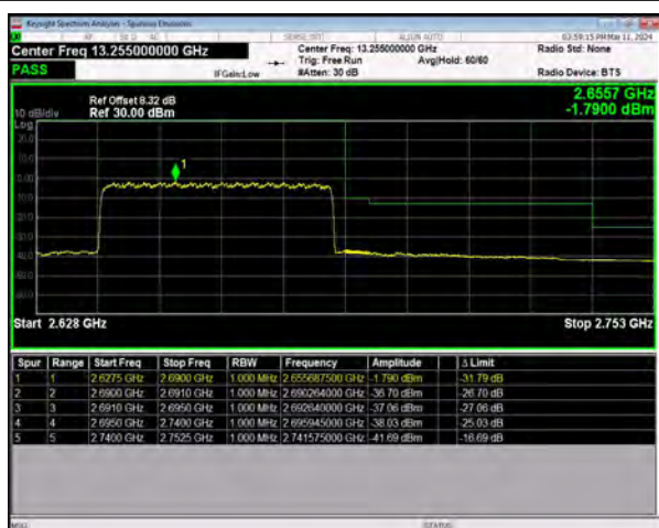
n41 SCS=30kHz DFT_QPSK BW=50MHz HighChannel=532998 RB=128@0
