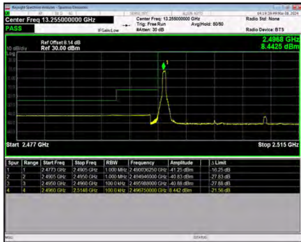
n41 SCS=30kHz DFT_QPSK BW=15MHz LowChannel=500700 RB=1@0
