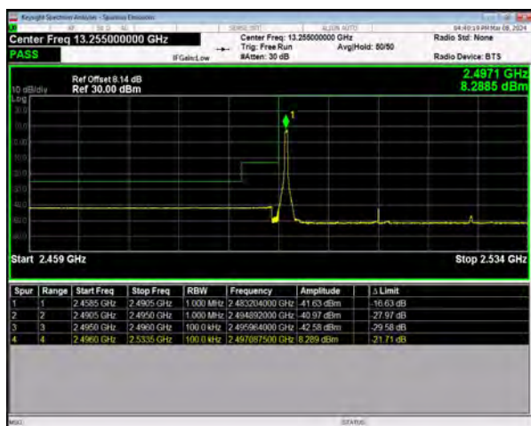
n41 SCS=30kHz DFT_16QAM BW=30MHz LowChannel=502200 RB=1@0
