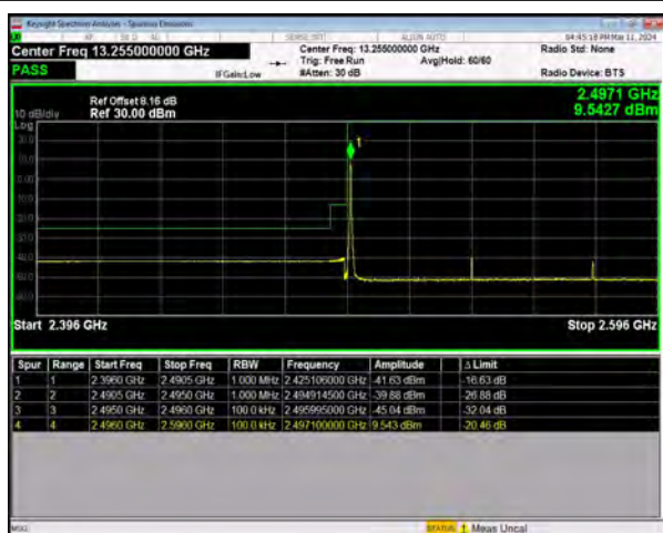
n41 SCS=30kHz DFT_BPSK BW=80MHz LowChannel=507204
