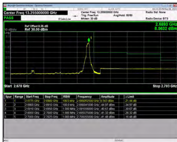
n41 SCS=30kHz DFT_16QAM BW=10MHz HighChannel=537000 RB=1@23
