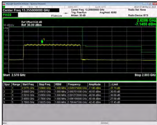
n41 SCS=30kHz DFT_64QAM BW=90MHz HighChannel=528996 RB=240@0
