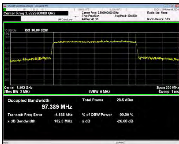
n41 SCS=30kHz CP_16QAM BW=100MHz Channel=518598 RB=273@0
