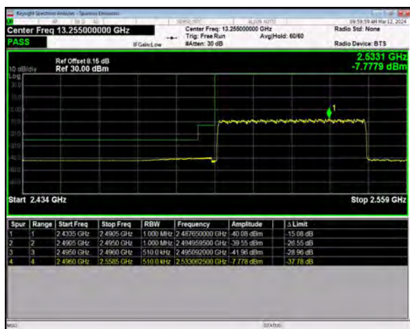
n41 SCS=30kHz CP_QPSK BW=50MHz LowChannel=504204 RB=133@0
