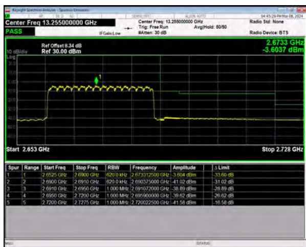
n41 SCS=30kHz DFT_16QAM BW=30MHz HighChannel=534996 RB=75@0
