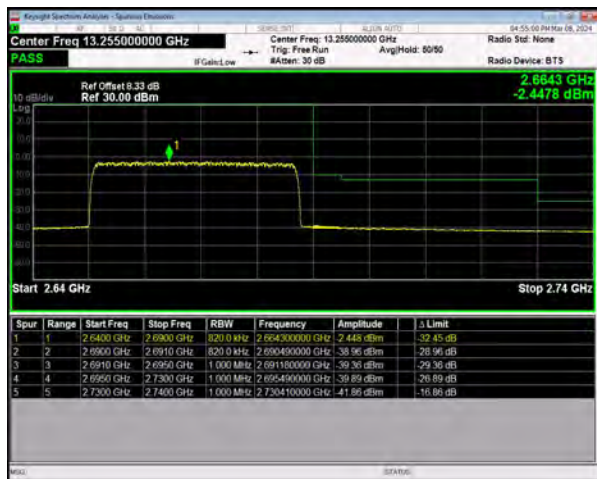
n41 SCS=30kHz DFT_16QAM BW=40MHz HighChannel=534000 RB=100@0
