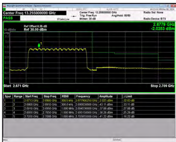
n41 SCS=30kHz DFT_BPSK BW=15MHz HighChannel=536496
