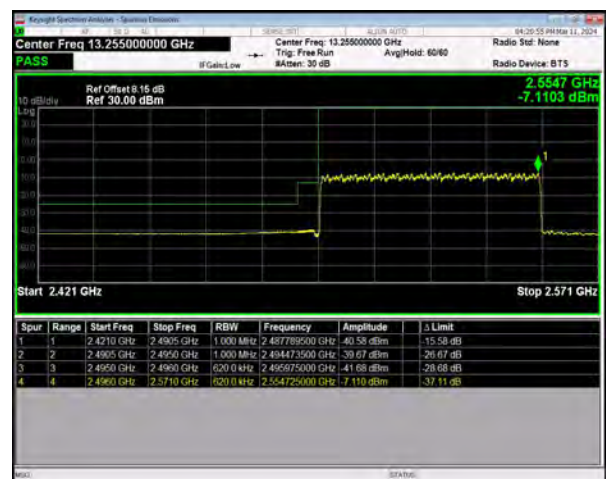
n41 SCS=30kHz DFT_16QAM BW=60MHz LowChannel=505200 RB=162@0
