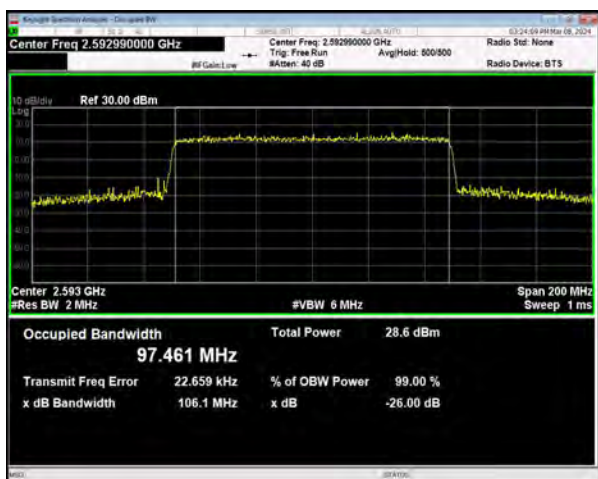
n41 SCS=30kHz CP_QPSK BW=100MHz Channel=518598 RB=273@0
