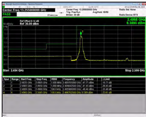
n41 SCS=30kHz DFT_256QAM BW=10MHz LowChannel=500202 RB=1@0
