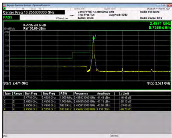
n41 SCS=30kHz DFT_BPSK BW=20MHz LowChannel=501204 RB=1@0
