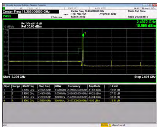
n41 SCS=30kHz DFT_QPSK BW=80MHz LowChannel=507204 RB=1@0
