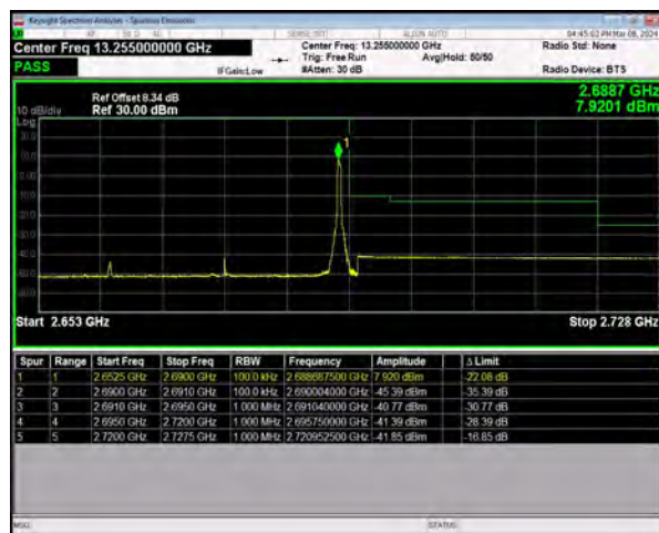
n41 SCS=30kHz DFT_16QAM BW=30MHz HighChannel=534996 RB=1@77
