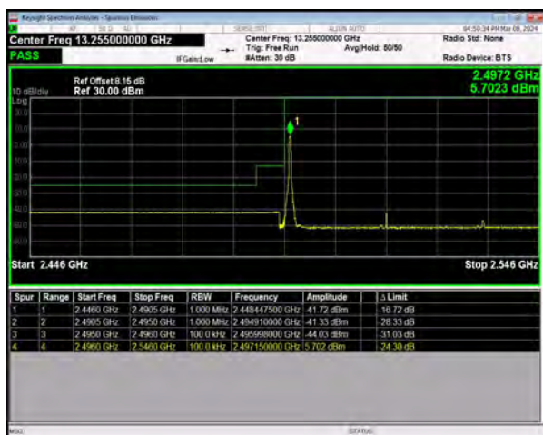
n41 SCS=30kHz DFT_64QAM BW=40MHz LowChannel=503202 RB=1@0
