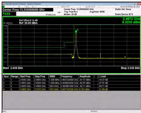
n41 SCS=30kHz DFT_QPSK BW=30MHz LowChannel=502200 RB=1@0
