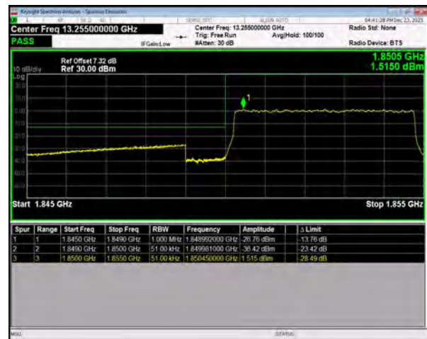
n25 SCS=15kHz DFT_256QAM BW=5MHz LowChannel=370500 RB=25@0
