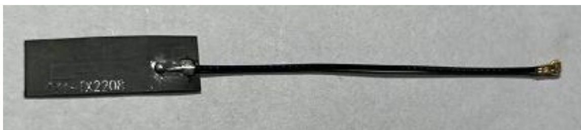
图 2 TYY-TX2208 WIFI Antenna finished product (with a length of 100mm and 3rd-generation terminals)
