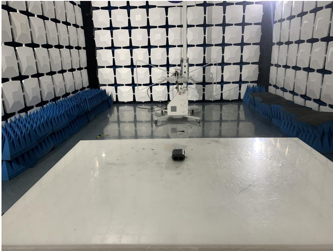
Below 1GHz for radiated emission test setup
