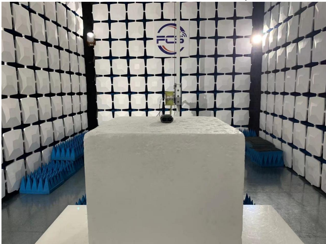
Above 1GHz for radiated emission test setup
