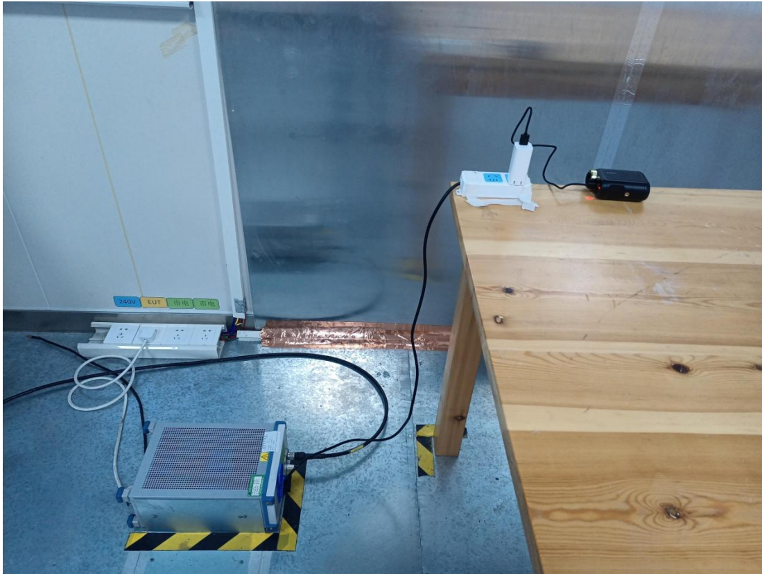
Conducted emission test setup
