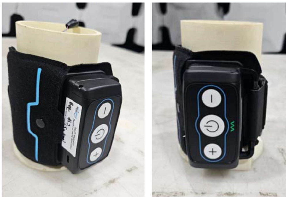
Picture # 4. Radiated emission test setup - Operation mode
