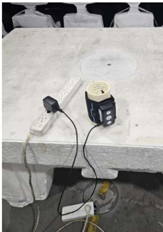
Picture # 5. Radiated emission test setup - Charging mode
