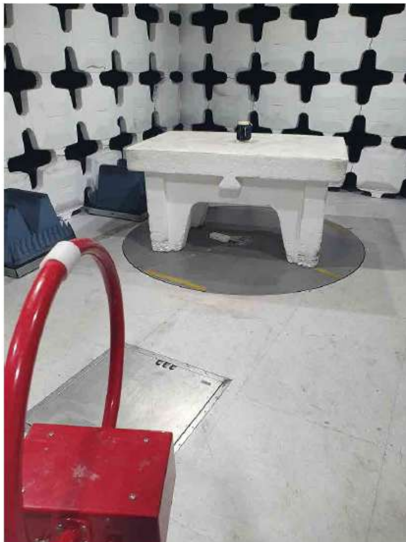
Picture # 6. Radiated Emission test setup below 30 MHz.
