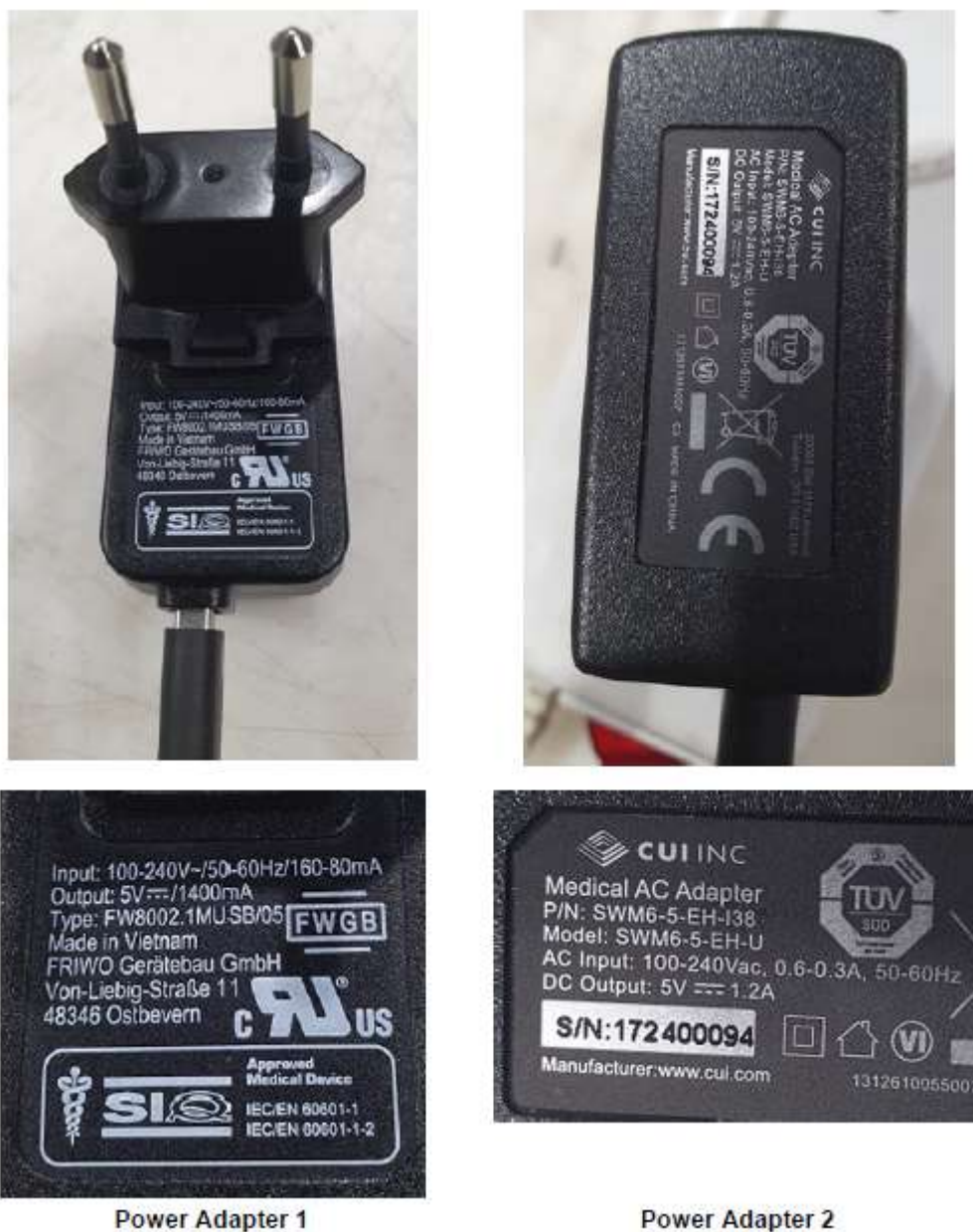
Figure 7 - Two Power Adapters used in tests. General view and ID label
