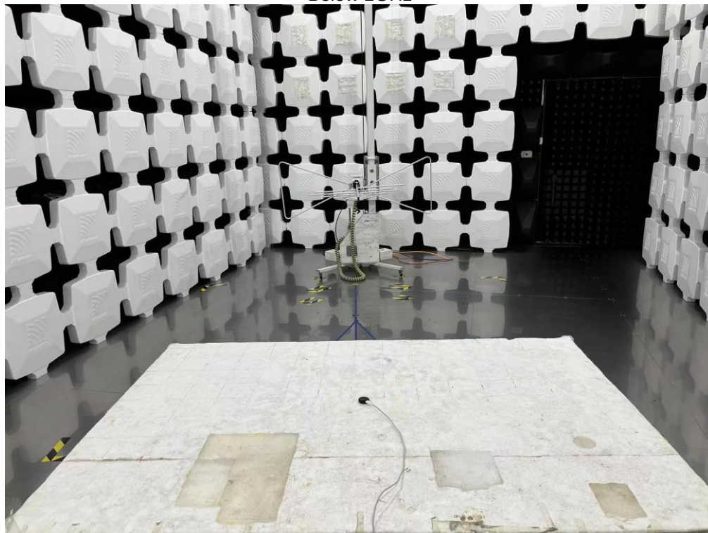
Radiated Spurious Emission Below 1GHz
