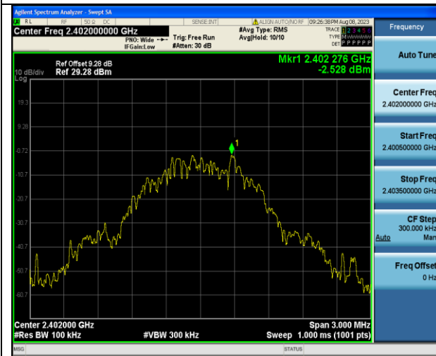
GFSK on Channel 00
