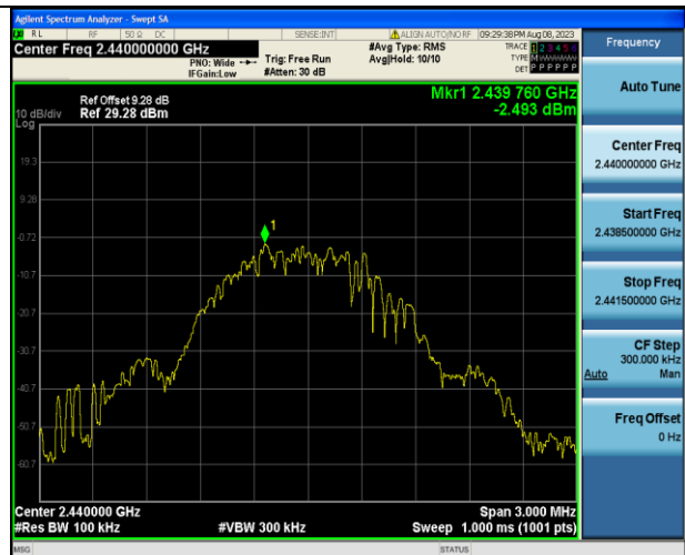
GFSK on Channel 19
