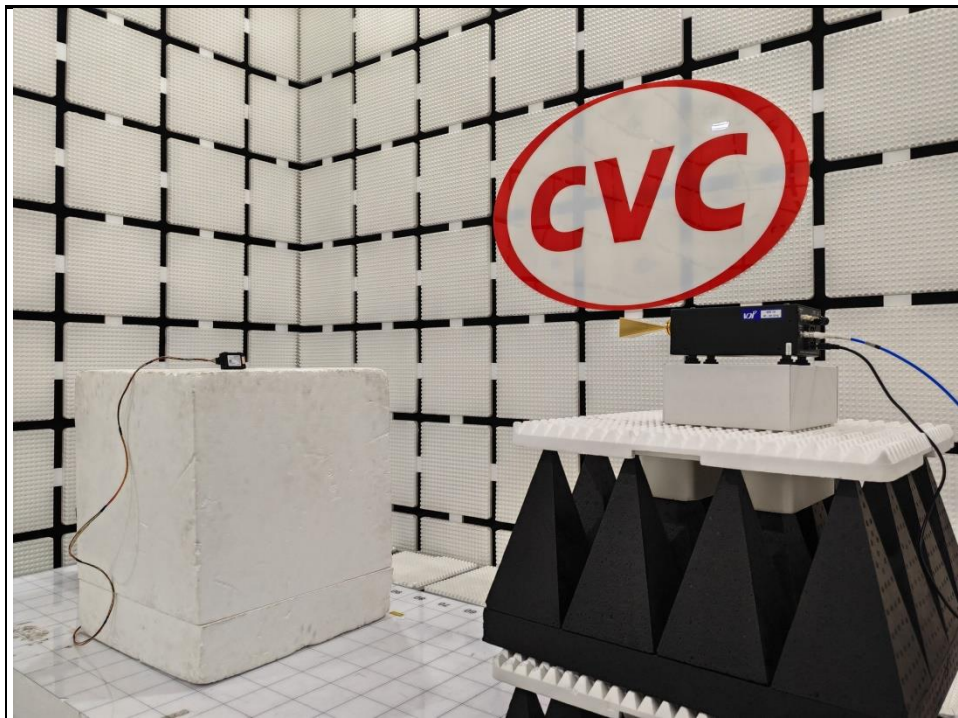
RADIATED EMISSION TEST (40GHz-200GHz)
