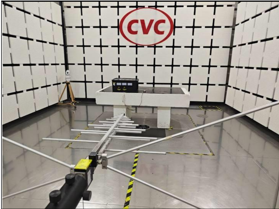
RADIATED EMISSION TEST (Below 1GHz)
