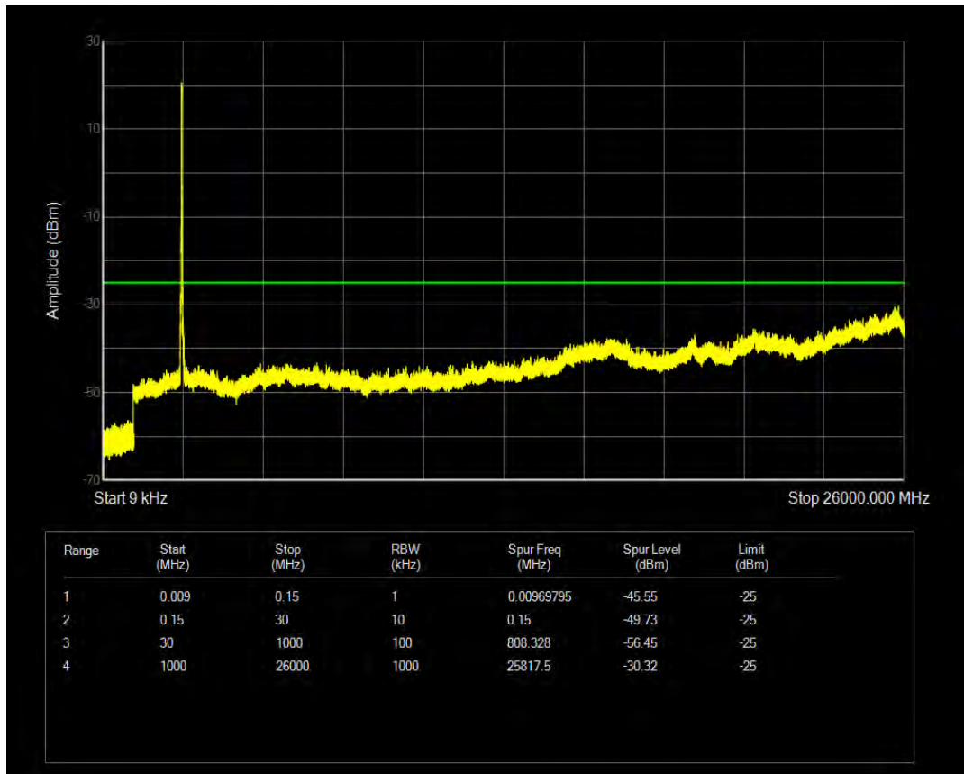
Band41(2555-2655) QAM16 BW=10MHz Channel=41190 RB Size=50 Position=#0
