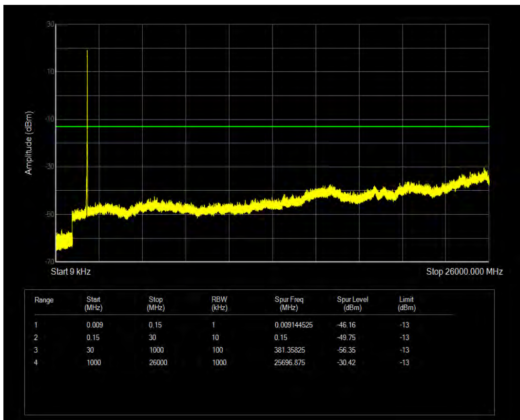
Band25 QPSK BW=20MHz Channel=26140 RB Size=100 Position=#0
