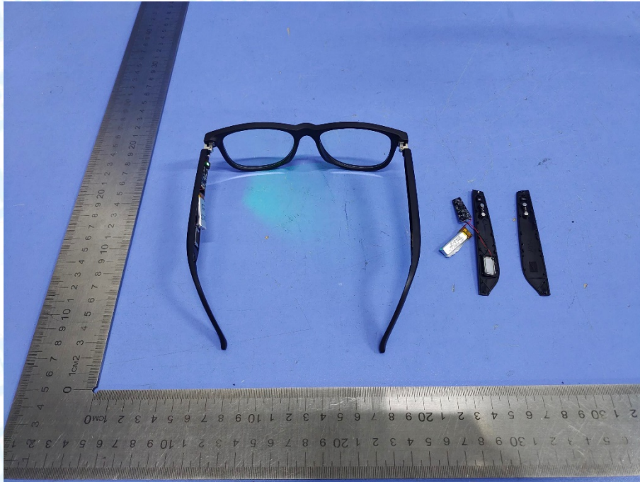
Photo 10 Appearance of PCB & Battery
