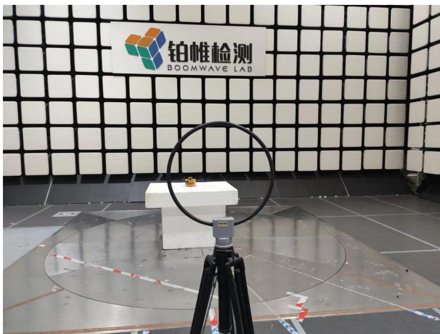
Spurious Radiated Emissions Test Setup (Below 30MHz)
