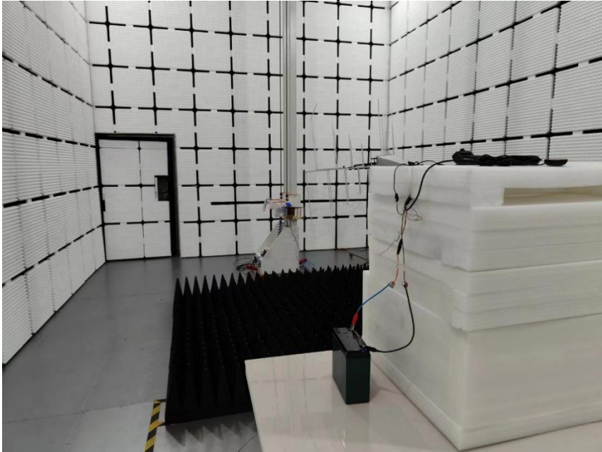
Radiated Emission Test Setup Photo - Above 1GHz
