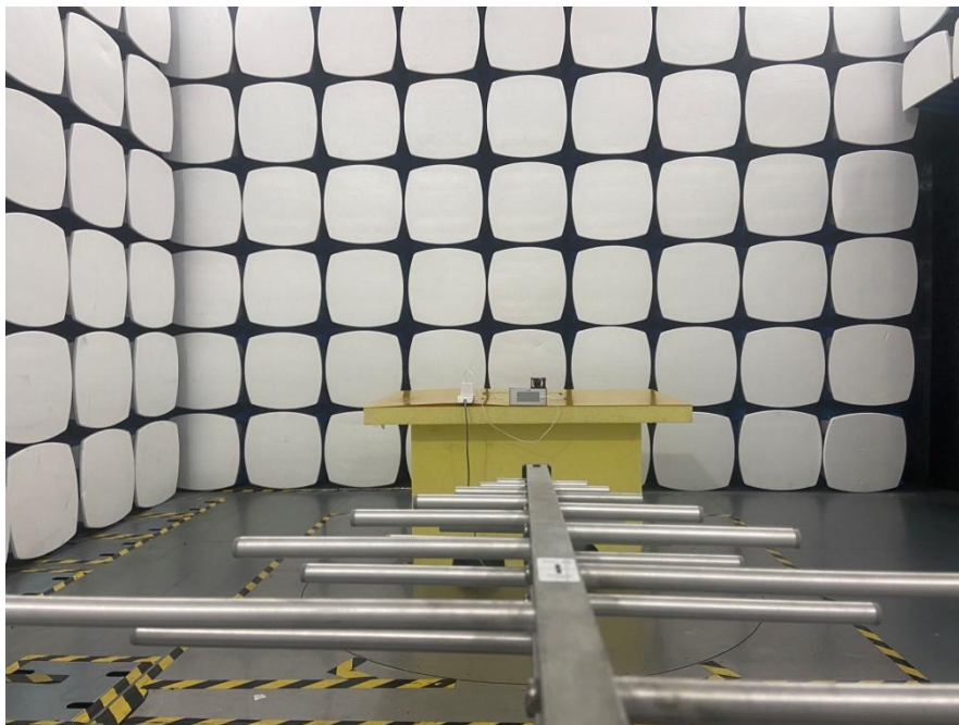
Radiated spurious emissions 30MHz to 1GHz for mode 2 to mode 5
