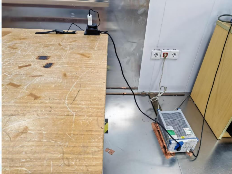
Photo of Setup for Radiated Emission (30MHz~1GHz)
