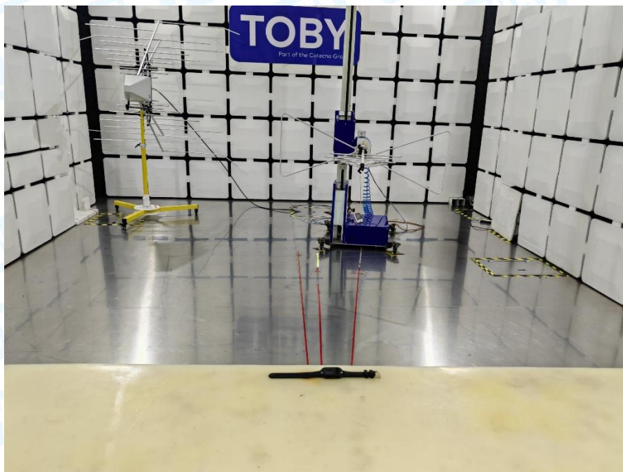
Photo of Setup for Radiated Emission (30MHz~1GHz)
