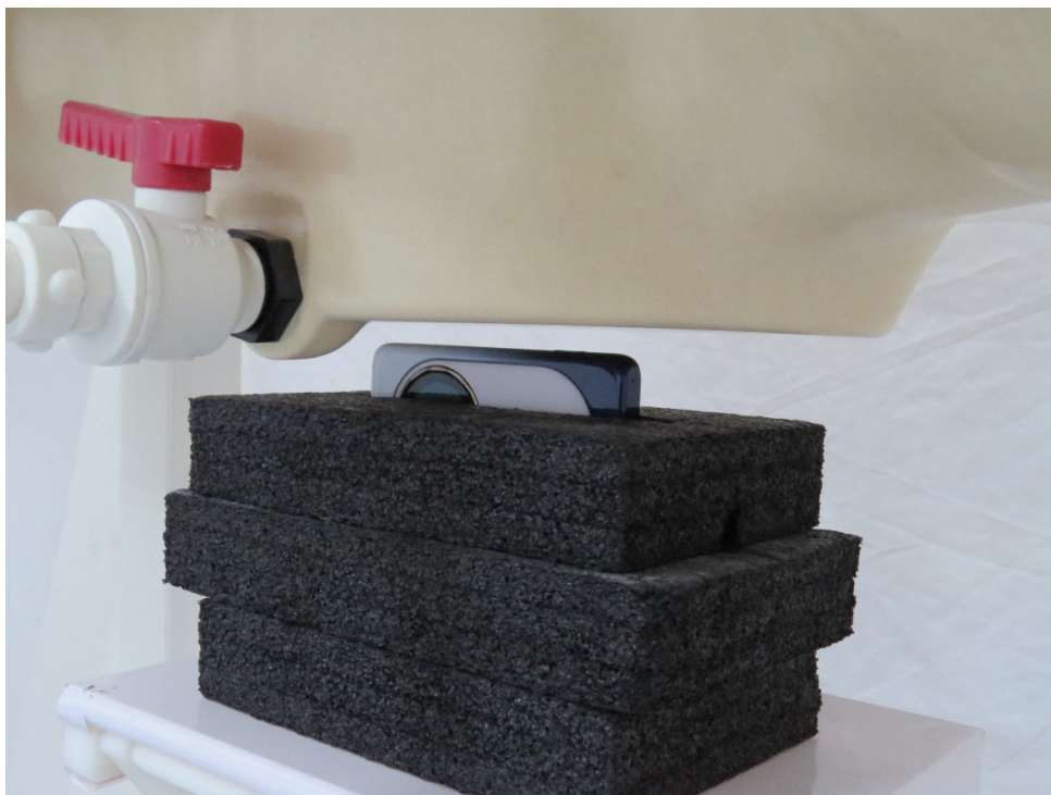
Picture 4: Right Edge, the distance from EUT to the bottom of the Phantom is 10mm
