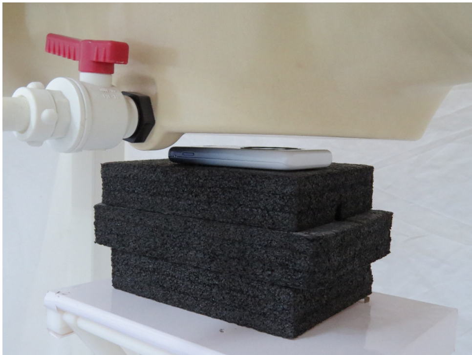
Picture 2: Front Side, the distance from EUT to the bottom of the Phantom is 10mm
