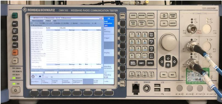
CMW 500 (2G/3G/4G Test Equipment)
