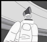
B. Tighten the sensor with tire valve
