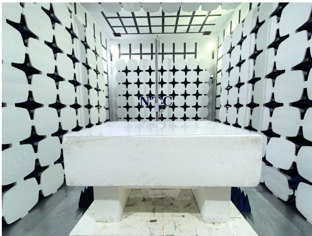
Photos of radiated emission test Above 1GHz
