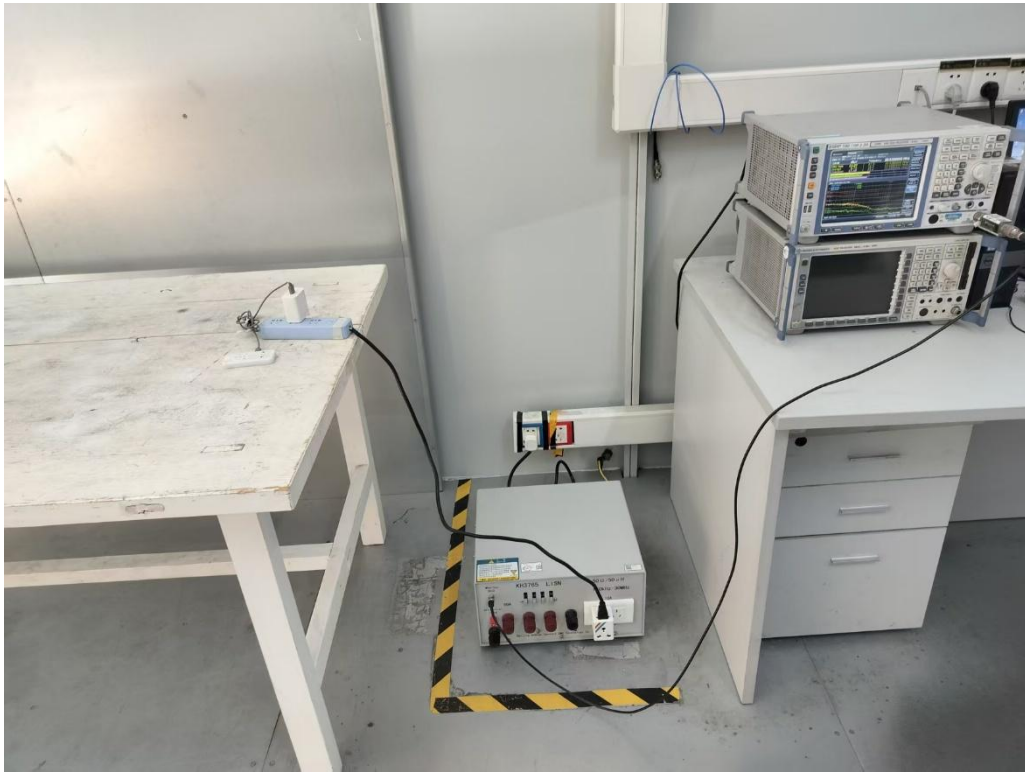
Photos of conducted emission test
