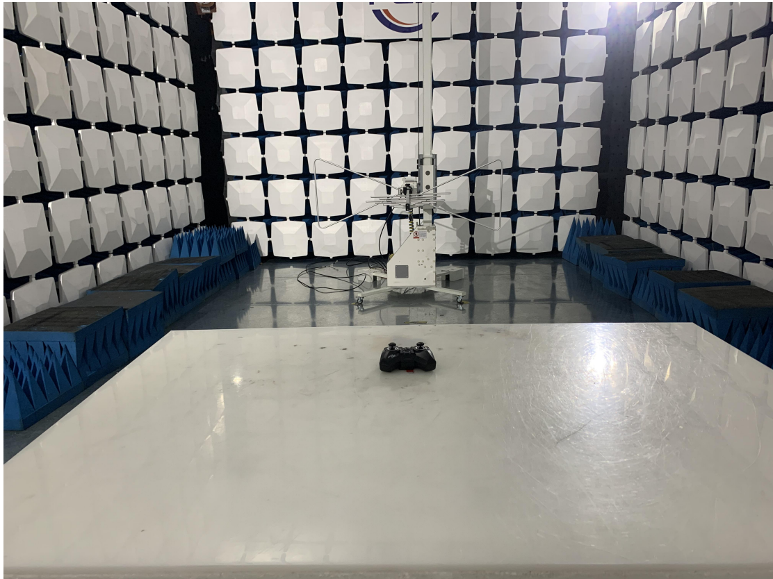
Above 1GHz for radiated emission test setup
