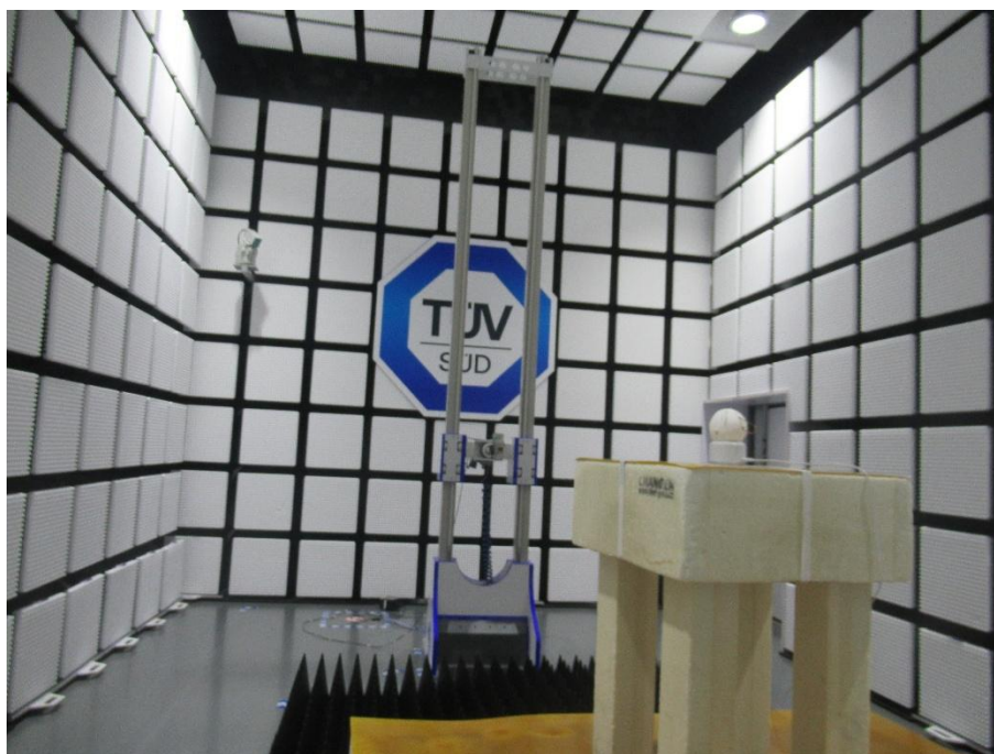
18GHz-40GHz RSE Setup
