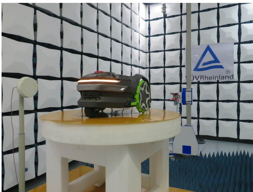
Photograph 2: Set-up photo for Radiated Spurious Emission, 1GHz - 18GHz
