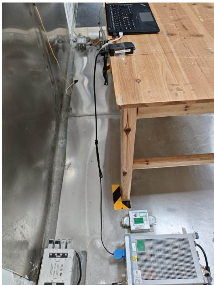
Conducted Emission Setup Side View
