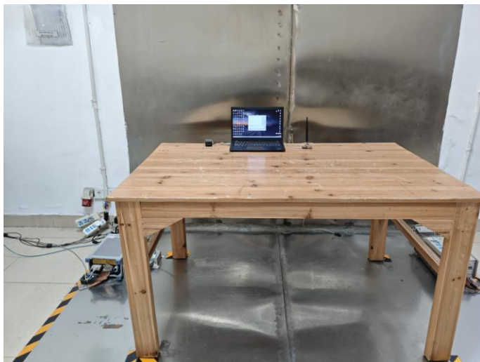
Conducted Emission Setup Front View
