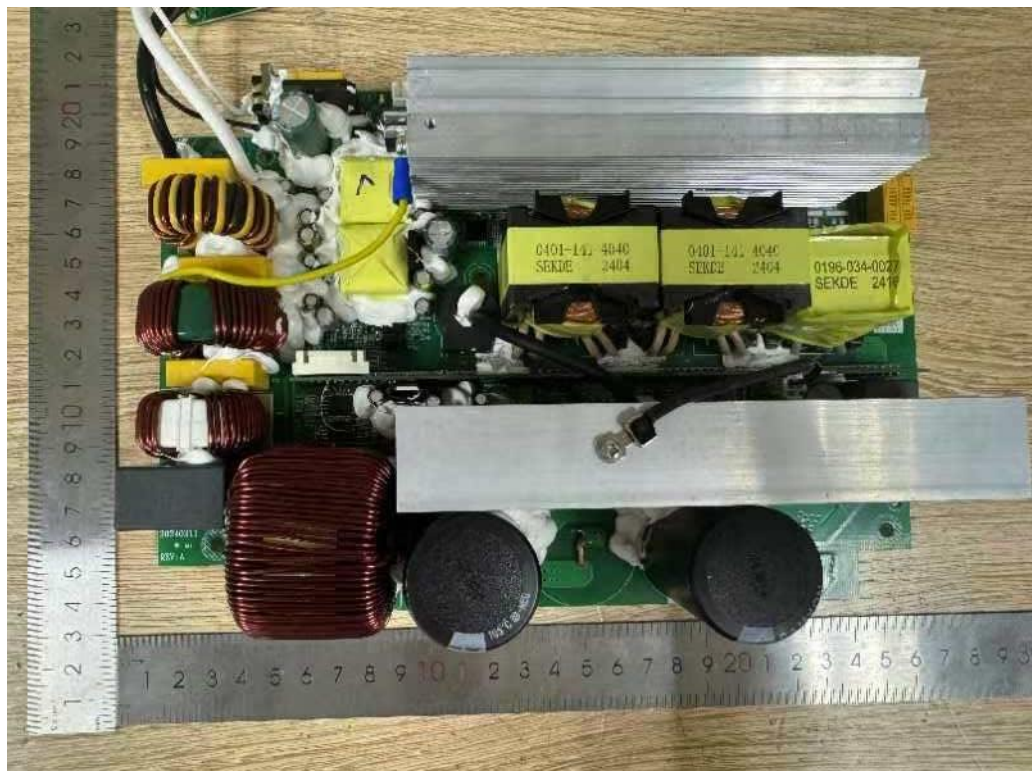
Figure 14 Top view of inverter board
