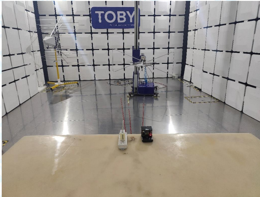
Photo of Setup for Radiated Emission (9kHz ~30MHz)
