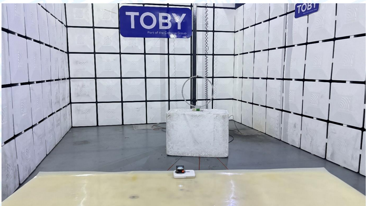
Photo of Setup for Radiated Emission (9kHz ~30MHz)
