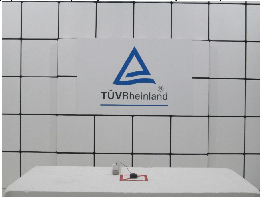
Photograph 8: Test Setup for Spurious Emissions (Back View 1)
