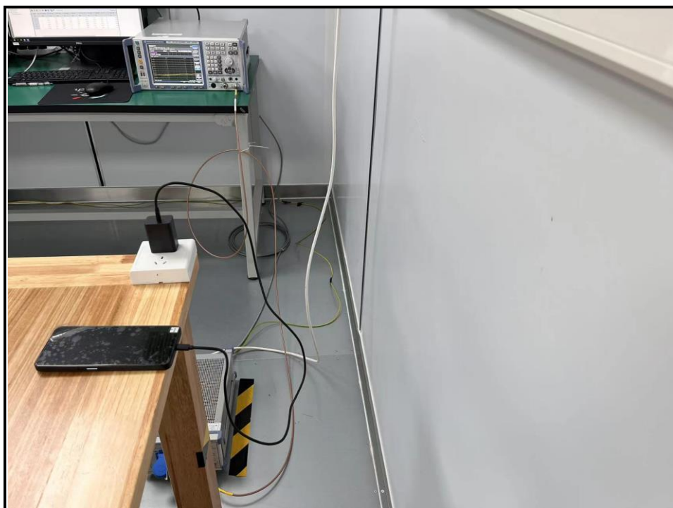
Fig. 4 Power line conducted emission setup photo
