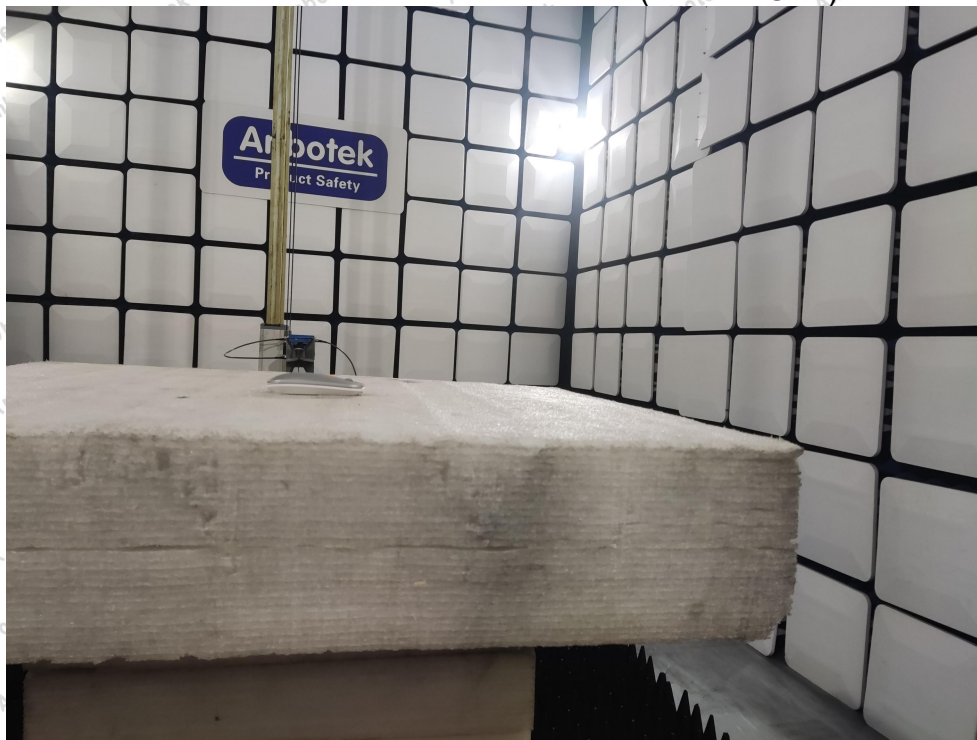
Photo of Radiation Emission Test (above 1GHz)
