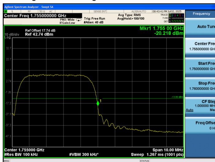
Higher Band Edge Plot on Channel 1513
