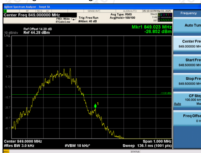
Higher Band Edge Plot on Channel 251
