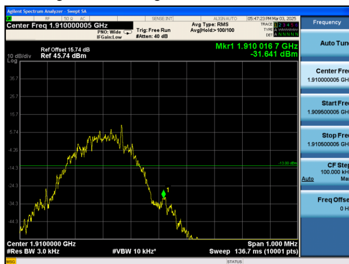
Higher Band Edge Plot on Channel 810
