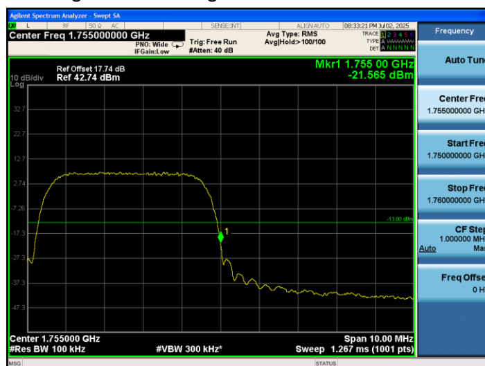
Higher Band Edge Plot on Channel 1513
