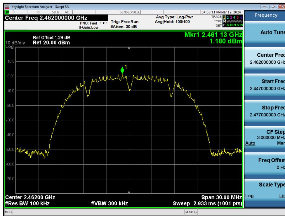
Band Edge NVNT b 2462MHz Ant1 Emission
