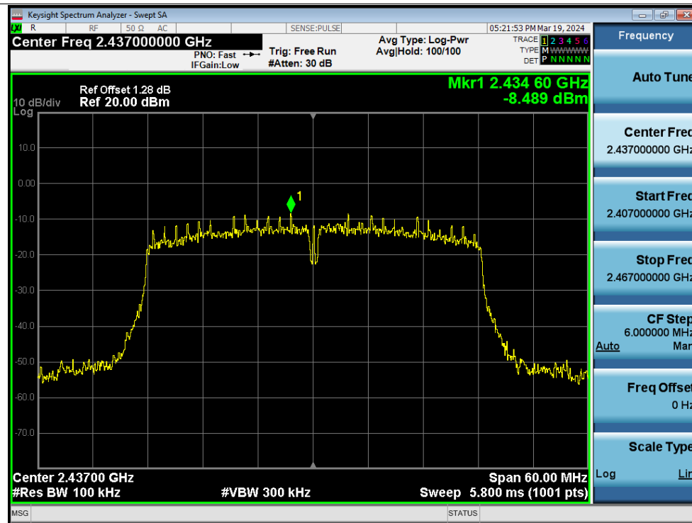
Tx. Spurious NVNT n40 2437MHz Ant1 Emission
