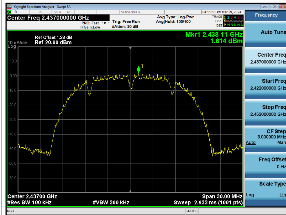
Tx. Spurious NVNT b 2437MHz Ant1 Emission
