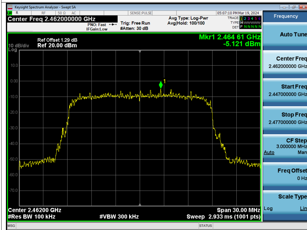
Tx. Spurious NVNT g 2462MHz Ant1 Emission
