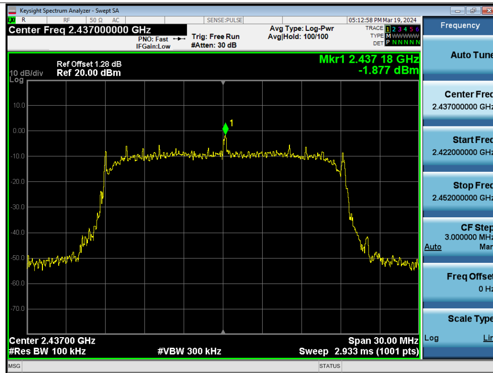
Tx. Spurious NVNT n20 2437MHz Ant1 Emission
