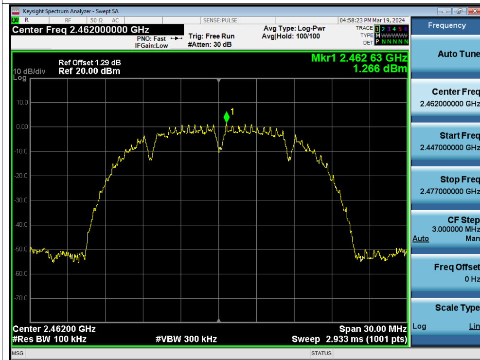
Tx. Spurious NVNT b 2462MHz Ant1 Emission
