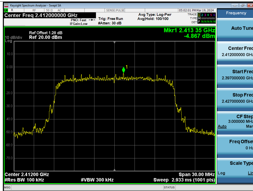
Tx. Spurious NVNT g 2412MHz Ant1 Emission
