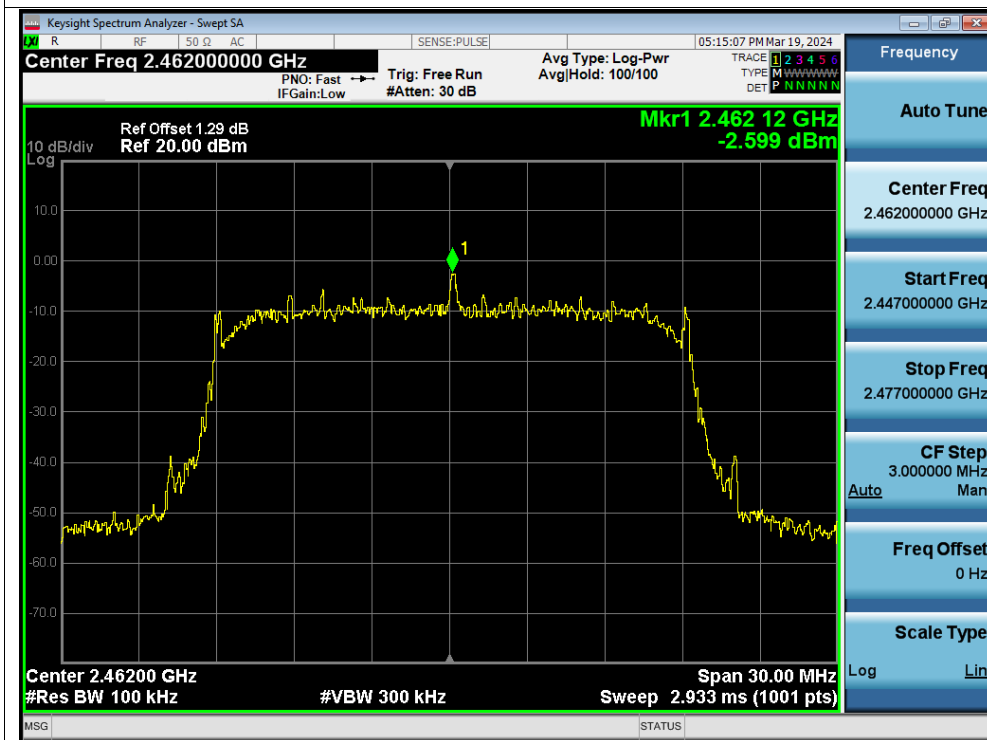
Band Edge NVNT n20 2462MHz Ant1 Emission
