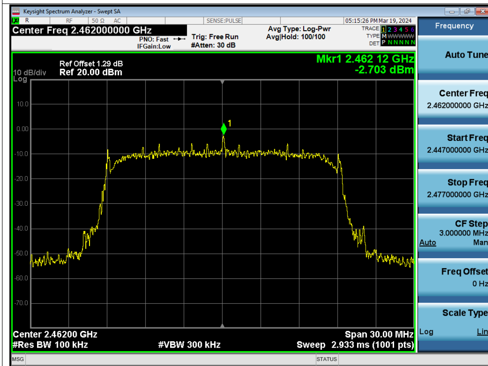
Tx. Spurious NVNT n20 2462MHz Ant1 Emission
