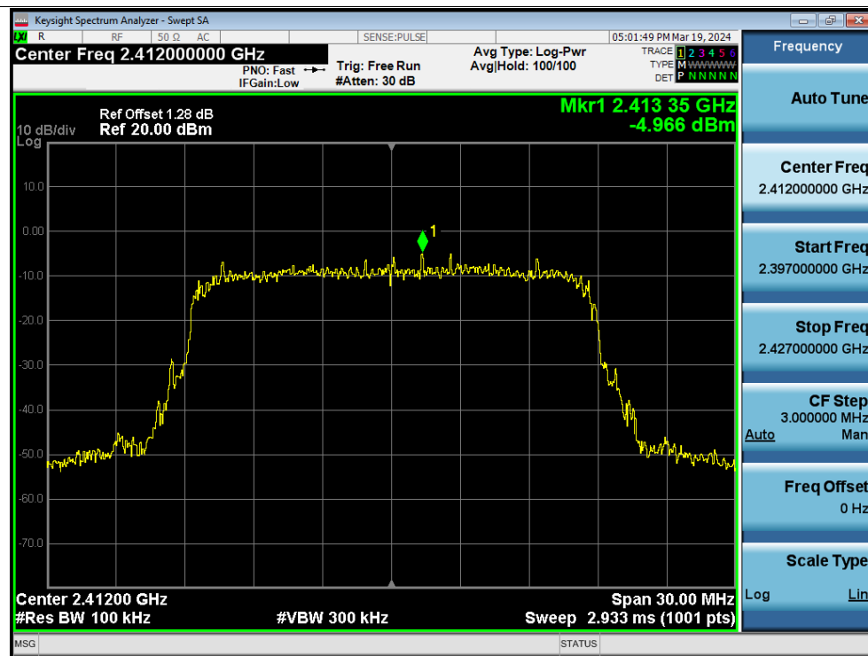
Band Edge NVNT g 2412MHz Ant1 Emission
