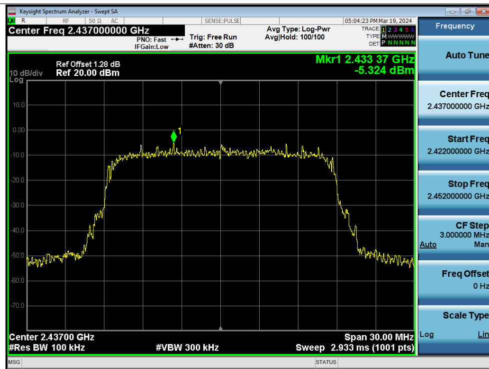
Tx. Spurious NVNT g 2437MHz Ant1 Emission
