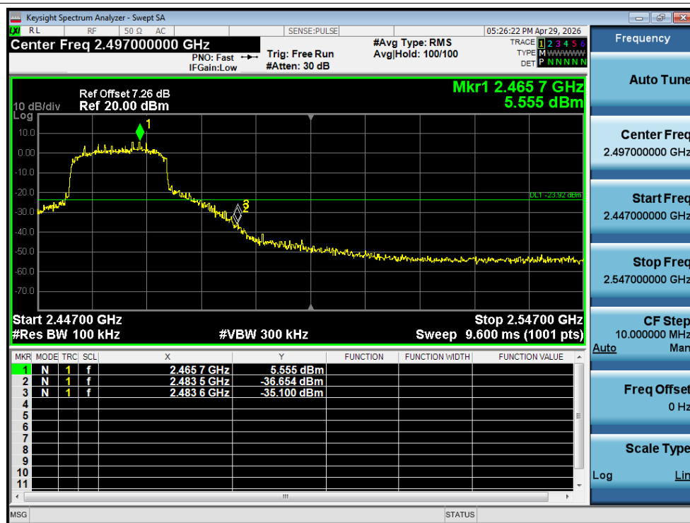
Band Edge NVNT g 2462MHz Ant1 Emission
