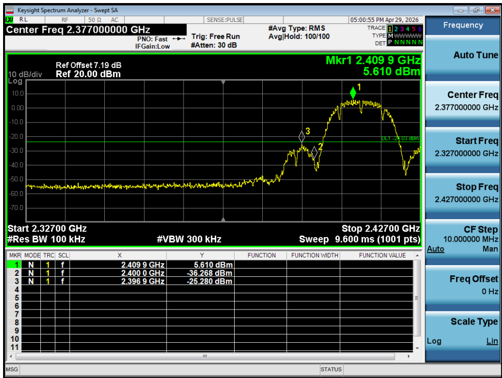
Band Edge NVNT b 2412MHz Ant1 Emission
