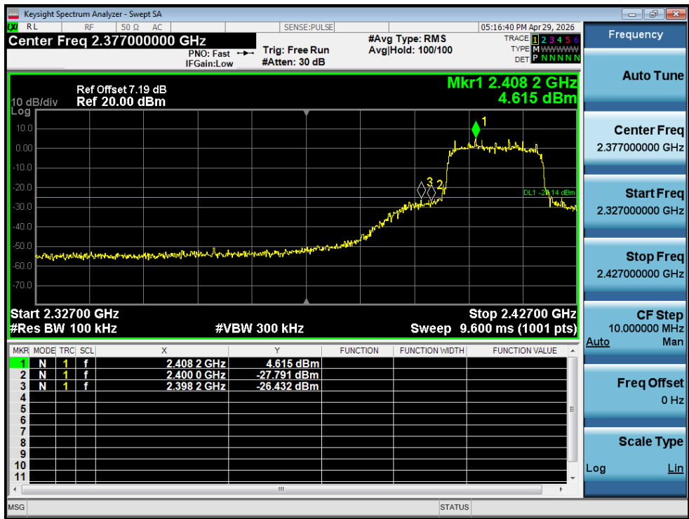
Band Edge NVNT g 2412MHz Ant1 Emission
