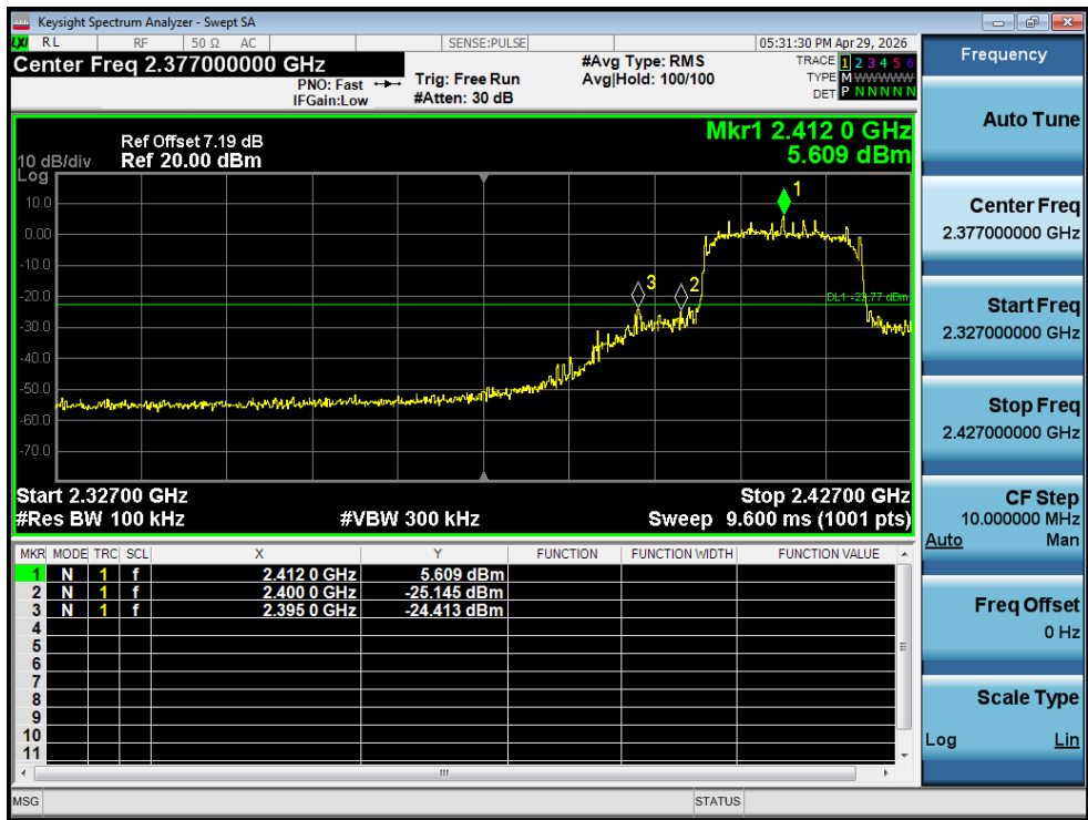
Band Edge NVNT n20 2412MHz Ant1 Emission
