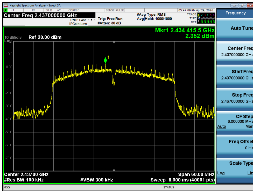
Tx. Spurious NVNT n40 2437MHz Ant1 Ref
