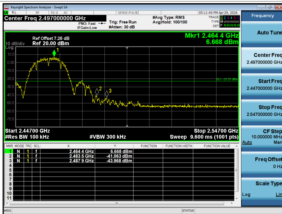
Band Edge NVNT b 2462MHz Ant1 Emission
