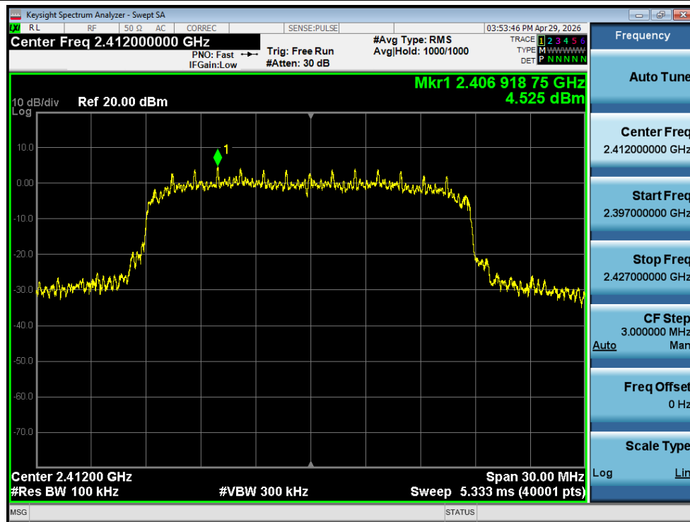
Tx. Spurious NVNT g 2412MHz Ant1 Ref
