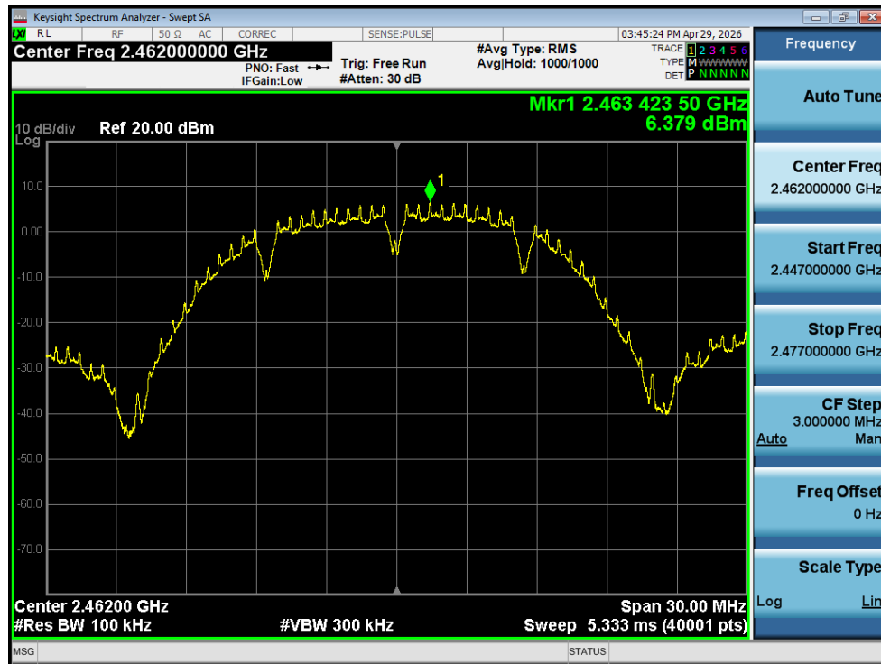
Tx. Spurious NVNT b 2462MHz Ant1 Ref
