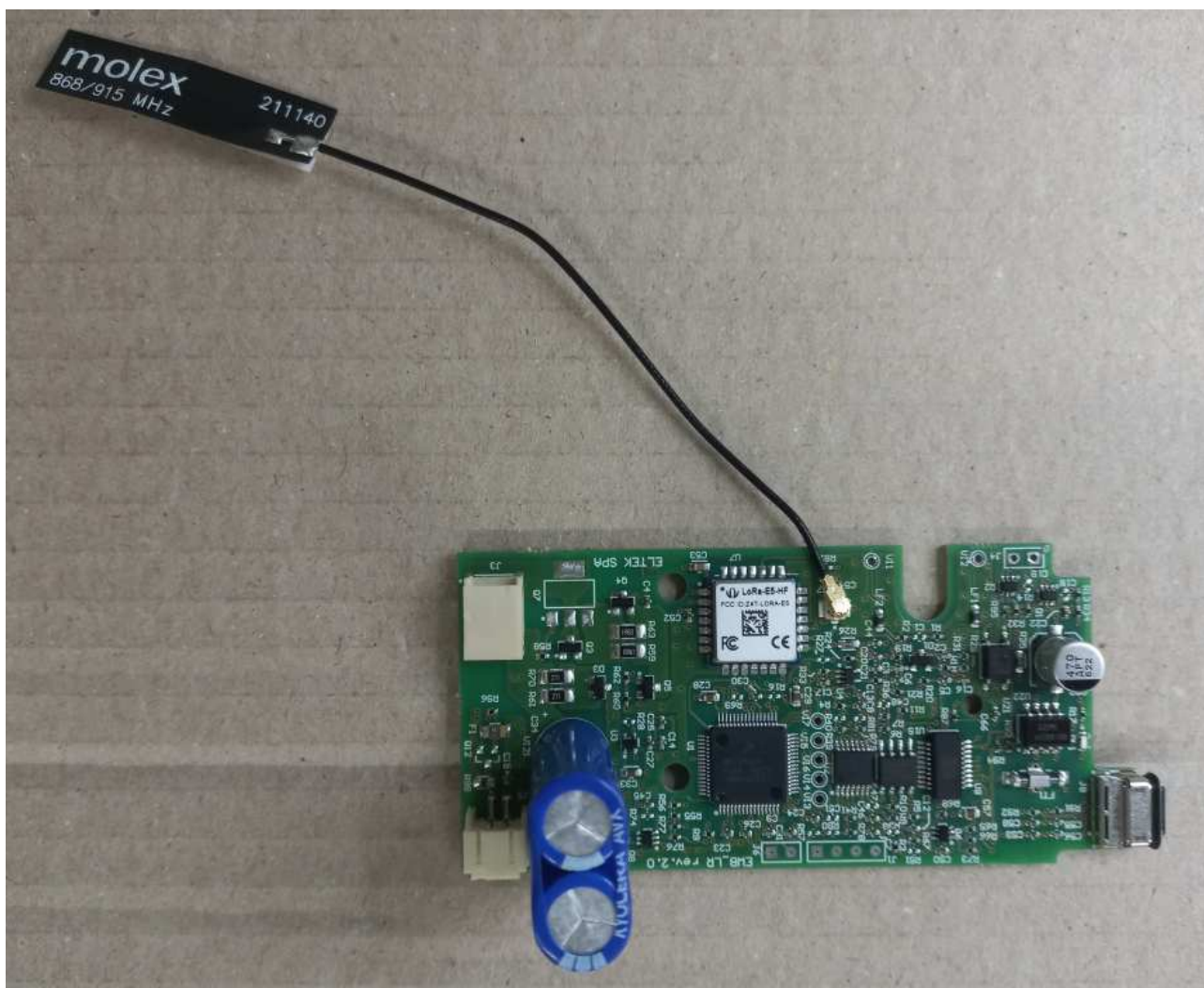
LoRa pcb and connected Molex antenna
