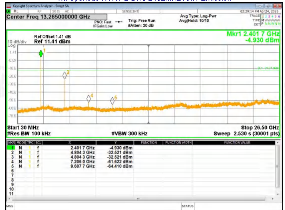
Tx. Spurious NVNT 2-DH5 2402MHz Ant1 Emission
