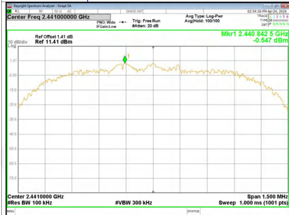
Tx. Spurious NVNT 3-DH5 2441MHz Ant1 Emission
