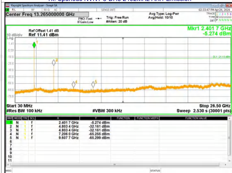
Tx. Spurious NVNT 3-DH5 2402MHz Ant1 Emission
