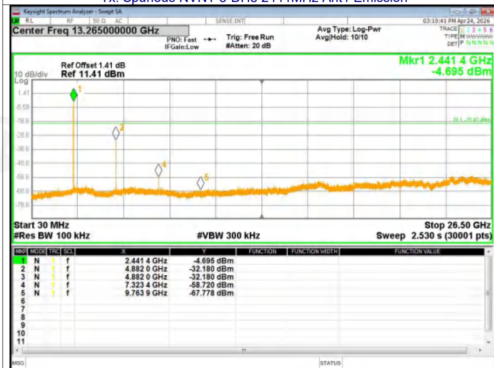
Tx. Spurious NVNT 3-DH5 2441MHz Ant1 Emission
