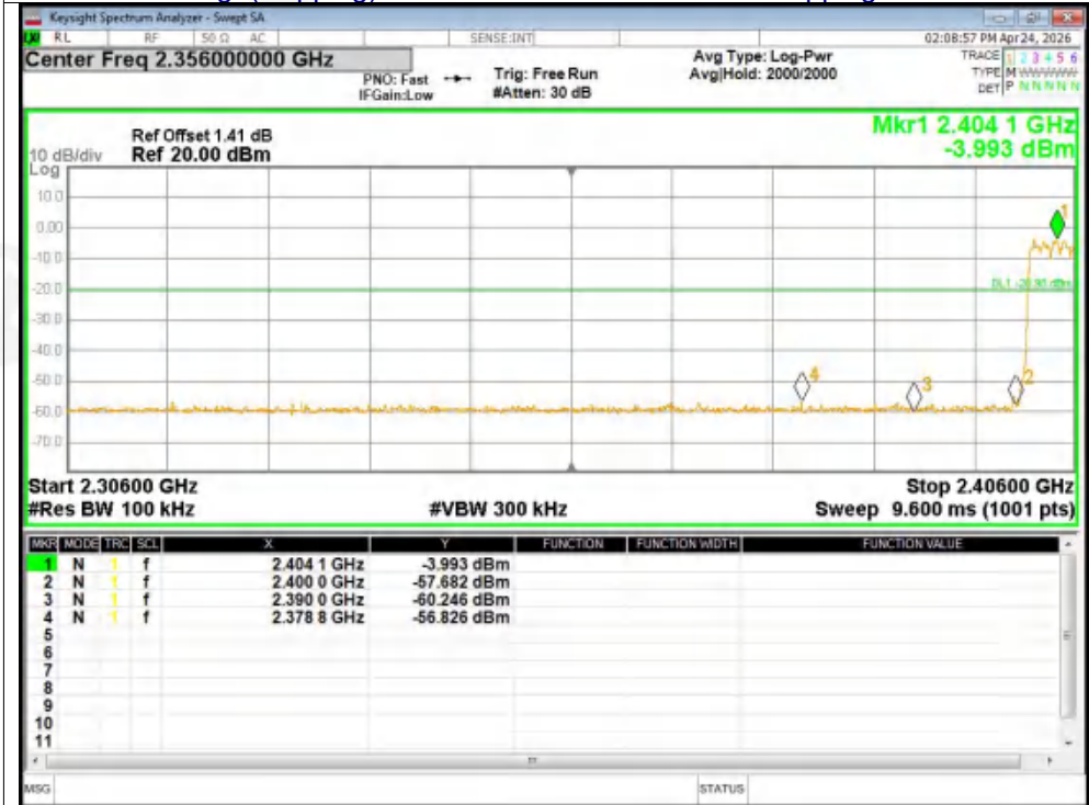
Band Edge(Hopping) NVNT 2-DH5 2402MHz Ant1 Hopping Emission
