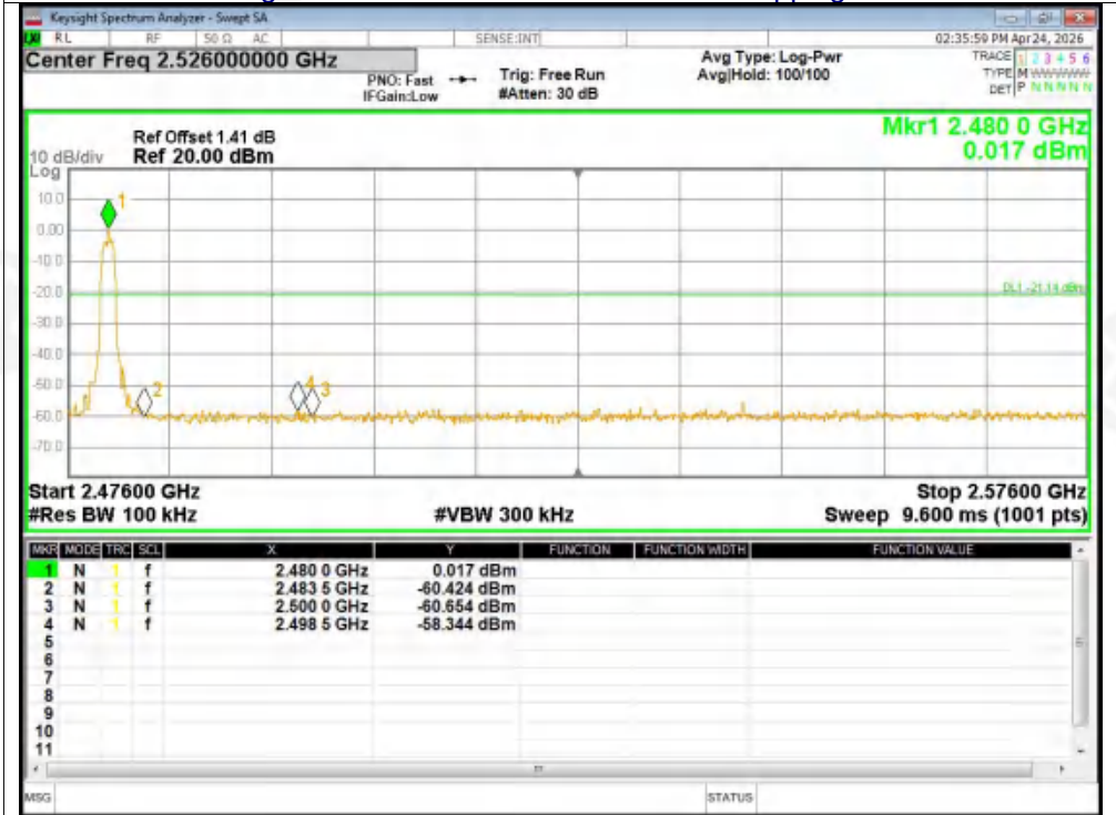
Band Edge NVNT 3-DH5 2480MHz Ant1 No-Hopping Emission
