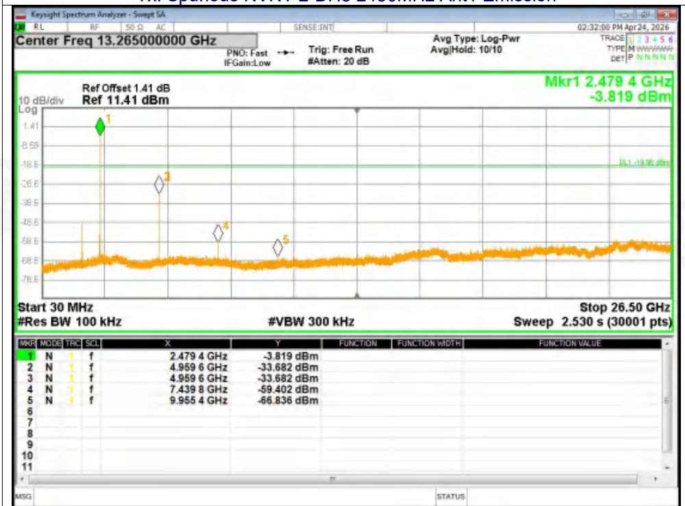
Tx. Spurious NVNT 2-DH5 2480MHz Ant1 Emission
