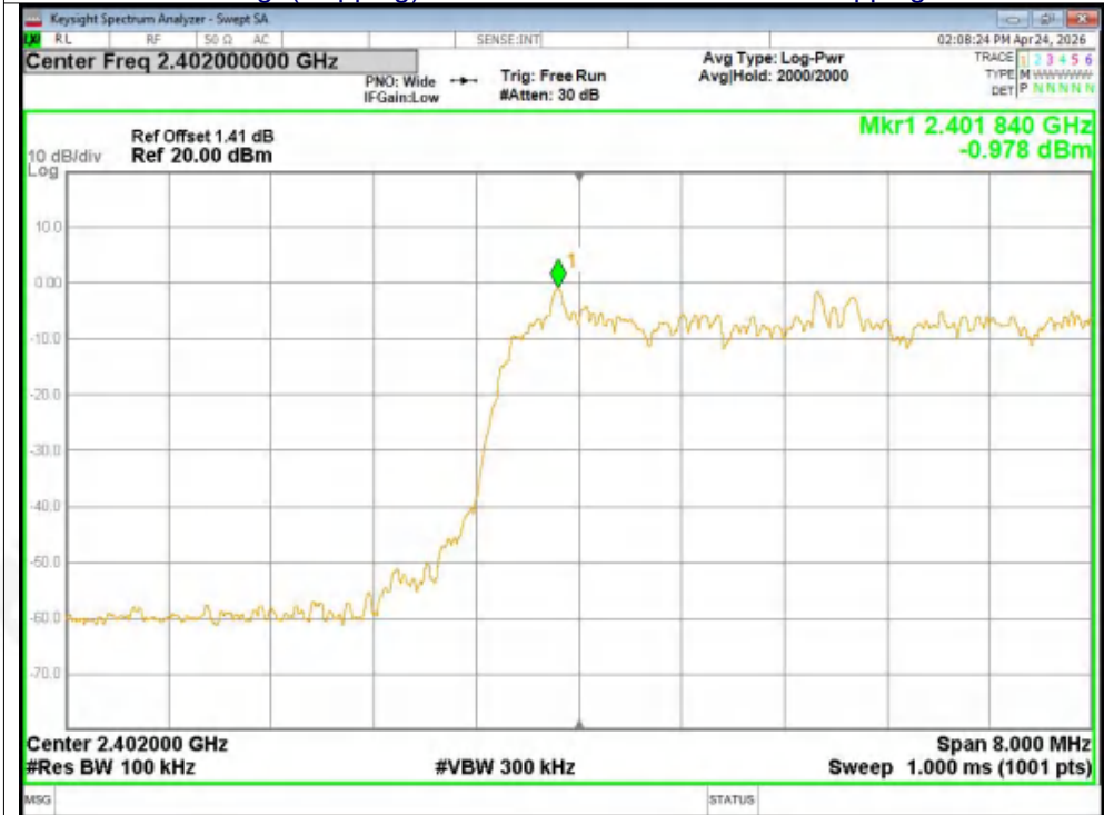
Band Edge(Hopping) NVNT 2-DH5 2402MHz Ant1 Hopping Emission
