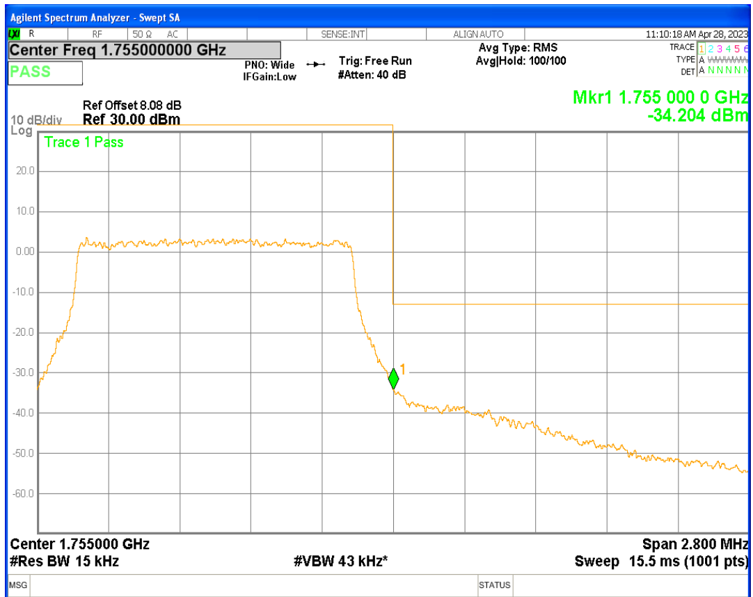
Band4 16QAM BW=10MHz Channel=20000 RB Size=50 Position=#0
