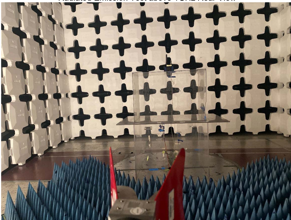
Radiated Emission Test above 1GHz Rear View
