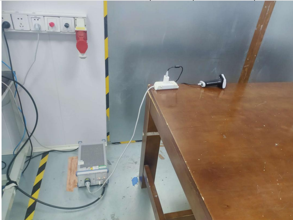
Conducted emissions at AC power line (150kHz-30MHz)
